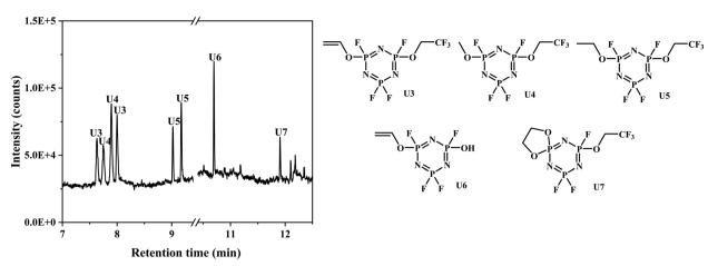
Fig. 7 Gas chromatogram obtained from sampling of extracted BE +  $CF_3$ PFPN electrolyte and the representation of the postulated structures of U3–U7 compounds.
