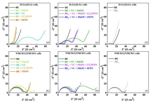
Fig. 9 (a)–(c) Nyquist plots of symmetric Si-Gr||Si-Gr cells assembled from galvanostatic cycled NMC811||Si-Gr cells; (d)–(f) Nyquist plots of symmetric NMC811||NMC811 cells assembled from harvested NMC811 and Si-Gr electrodes.
