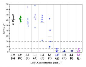
Fig. 3 SET values of electrolytes containing LiPF<sub>6</sub> in different concentrations: (a) BE, (b) BE + VC + PhEPi, (c-i) different molar concentrations of LiPF<sub>6</sub> in EC:EMC 3:7 vol + 5% PFPN + 8% VC + 0.038 M PhEPi and (j) 1.5 M LiPF6 in EC: EMC 3:7 vol + 5% CF<sub>3</sub>PFPN + 8% VC + 0.038 M PhEPi.
