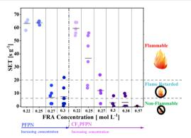
Fig. 2 SET values determined for electrolyte compositions containing different concentrations of PFPN and CF<sub>3</sub>PFPN in BE (EC:EMC 3:7 vol + 1.0 M LiPF<sub>6</sub>) + 0.038 M PhEPi + 8% VC. Details on the sample number are summarized in Table 1.
