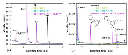
Fig. 6 (a) Gas chromatograms obtained from 10 s SPME sampling of extracted BE or electrolyte containing PhEPi, PhEPi + VC or PhEPi + VC + CF<sub>3</sub>PFPN. (b) Gas chromatograms obtained from 600 s SPME sampling of extracted BE or electrolyte containing PhEPi, PhEPi + VC or PhEPi + VC + CF<sub>3</sub>PFPN. The postulated structures of the compounds are represented in the figures at the retention time of the corresponding peaks.
