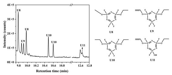
Fig. 8 Gas chromatogram obtained from sampling of extracted BE + PFPN electrolyte and the representation of the postulated structures of U8–U11 compounds.
