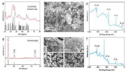
Fig. 1 Preparation and characterization of the Cu<sub>2</sub>(OH)<sub>3</sub>Br and pure Cu catalysts. (a) XRD pattern, (b) SEM image and (c) XPS pattern of Cu<sub>2</sub>(OH)<sub>3</sub>Br. (d) XRD pattern, (e) SEM images and the (f) XPS pattern of the pure Cu catalyst.
