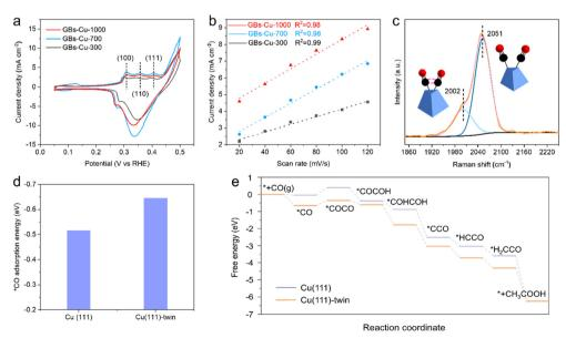
Fig. 3 (a) OH<sup>-</sup> adsorption spectral measurements and (b) double layer capacitance comparison of GBs-Cu-x (x represents 300, 700 and 1000). (c) In situ Raman spectroscopy of GBs-Cu-300 under CO electrolysis at -1.3 V versus Ag/AgCl. (d) \*CO adsorption energy on Cu(111) and the Cu(111)twin. (e) The energy profiles towards acetate formation on Cu(111) and the Cu(111)-twin.
