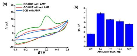
Fig. 2 (a) CVs of AMP with several electrodes: GCE, rGO/GCE; (b) the relationship of the AMP peak current with the quantity of electrode modifier: 2.5, 5.0, 7.5, 10.0 and 12.5  $\mu$ g ( $C_{AMP} = 10 \mu$ M in BRBS 0.2 M, pH 6.0).
