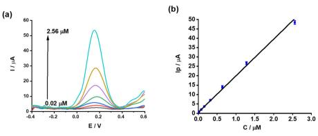
Fig. 4 (a) DPVs of AMP at several concentrations: 0.02, 0.08, 0.16, 0.32, 0.64, 1.28, 2.56  $\mu$ M. (b) The plot of  $I_p$  versus  $C_{AMP,\mu M}$ .
