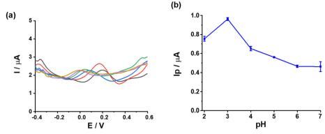
Fig. 3 (a) DPV curves of AMP with various pH values: 2, 3, 4, 5, 6 and 7; (b) plot of I<sub>D</sub> and pH.
