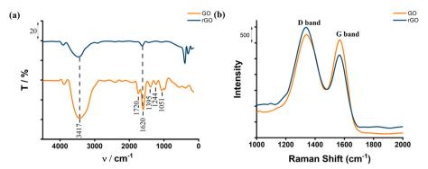
Fig. 1 (a) FT-IR of GO and rGO; (b) Raman spectra of GO and rGO.
