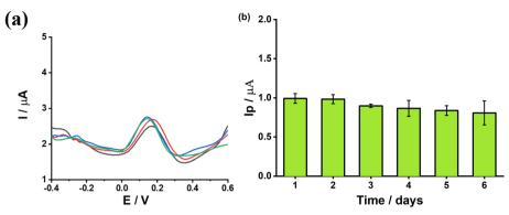
Fig. 6 (a) Reproducibility of AMP 0.02  $\mu$ M in BRBS pH 3 with 4 times conductive electrode modifications, (b) peak current ( $I_p$ ) variations of AMP across six successive modifications of rGO/GCE.
