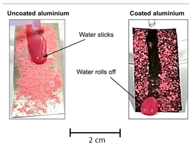
**Fig. 9** Optical images showing the self-cleaning behavior of uncoated and tetradecanoic acid-coated aluminium surfaces. Dust particles remain adhered to the uncoated surface, whereas water droplets roll off the coated surface with effectively removing the dust and demonstrating the self-cleaning effect.
