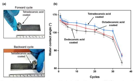
Fig. 7 (a) Optical images of the sandpaper abrasion test for examining the durability of the coating and (b) WCA vs. sandpaper abrasion cycle plot for coated surfaces.
