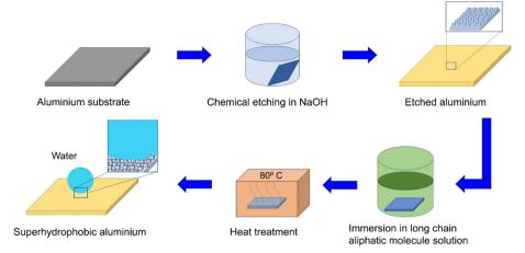
Fig. 1 Schematic diagram for the preparation of the superhydrophobic aluminium surface using long-chain fatty acids by a simple immersion technique
