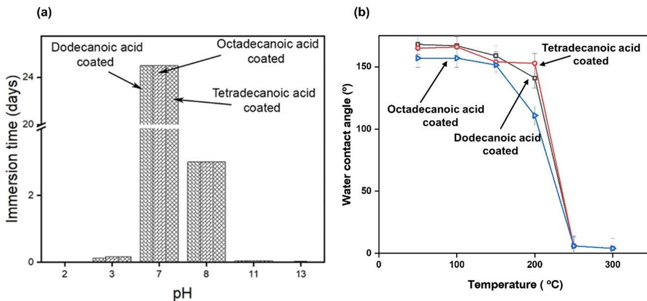
**Fig. 8** (a) Samples immersed in solutions of varying pH levels retained their superhydrophobicity, demonstrating good chemical stability. (b) Water contact angle vs. temperature plot for all coated aluminium after 2 h of annealing, showing thermal stability of the coated samples.
