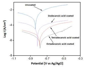
Fig. 10 Potentiodynamic polarization curves for uncoated and different long-chain fatty acid coated superhydrophobic aluminium surfaces in 3.5% (w/v) NaCl solution.
