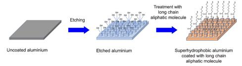
Fig. 3 Schematic representation of the reaction mechanism on the aluminium substrate after etching and testing by aliphatic molecules.
