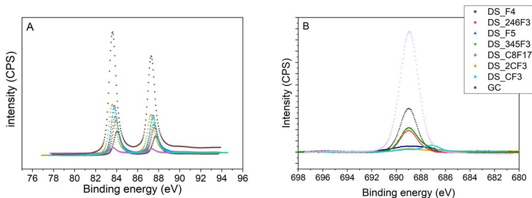
Fig. 8 (A) Au<sub>4f</sub> and (B) F<sub>1s</sub> core level spectra of Au thin film before and after modification by electrochemical reduction with various aryldiazonium salts.
