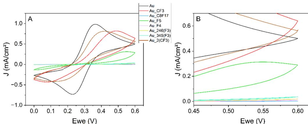
Fig. 9 (A) Cyclic voltammograms at a scan rate of 50  $\text{mV s}^{-1}$  for gold electrodes in a 5 mM  $\text{Fe}(\text{CN})_6^{3-/4-}$  solution before and after deposition of different diazonium salts: **DS\_CF3** (red); **DS\_C8F17** (blue); **DS\_F5** (green); **DS\_F4** (pink); **DS\_246(F3)** (orange); **DS\_345(F3)** (cyan); and **DS\_2(CF3)** (brown) and (B) its zoom.
