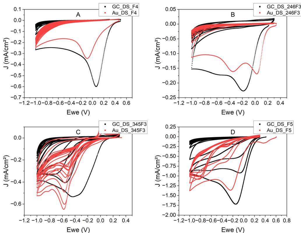
**Fig. 2** Cyclic voltammograms recorded at a sweep rate of  $100 \text{ mV s}^{-1}$  on GC (black) and gold (red) electrodes in 1 mM solutions of 4 salts: **DS\_F4** (A), **DS\_246(F3)** (B), **DS\_345(F3)** (C), and **DS\_F5** (D). The salts were dissolved in an *n*-NBu<sub>4</sub>PF<sub>6</sub>/ACN electrolyte. All potentials are reported versus an Ag/Ag<sup>+</sup> reference electrode, with a platinum gauze as counter electrode.
