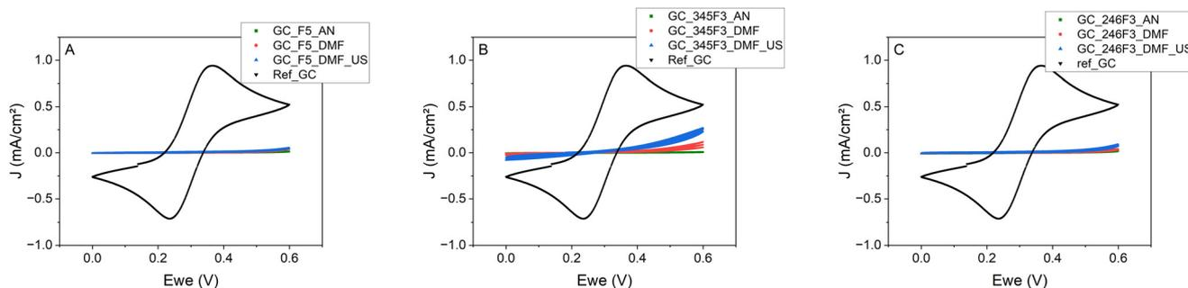
Fig. 3 Cyclic voltammograms at a scan rate of  $50 \text{ mV s}^{-1}$  for **DS\_F5** (A), **DS\_345(F3)** (B) and **DS\_246(F3)** (C) grafting on GC electrodes before and after different baths in acetonitrile (red), DMF (green), and DMF + ultrasonic bath for 2 minutes (blue) in a  $5 \text{ mM Fe(CN)}_6^{3-/4-}$  solution.
