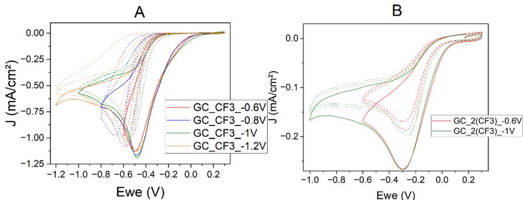
Fig. 5 Cyclic voltammograms recorded at a sweep rate of  $100 \text{ mV s}^{-1}$  on GC electrode in solutions of  $1 \text{ mM}$  of DS\_CF3 (A) and DS\_2(CF3) (B) until different potential:  $-0.6 \text{ V}$  (red),  $-0.8 \text{ V}$  (blue),  $-1 \text{ V}$  (green) and  $-1.2 \text{ V}$  vs.  $\text{Ag}/\text{Ag}^+$  (orange). The first cycle is shown as a solid line, while cycles 2 and 3 are represented with dashed lines.
