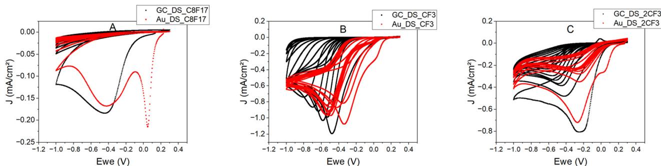
Fig. 4 Cyclic voltammograms recorded at a sweep rate of  $100 \text{ mV s}^{-1}$  on GC (black) and gold (red) electrodes in  $1 \text{ mM}$  solutions of DS\_C8F17 (A), DS\_CF3 (B), and DS\_2(CF3) (C) salts. The salts were dissolved in a  $n\text{-NBu}_4\text{PF}_6/\text{ACN}$  electrolyte. All potentials are reported versus an Ag/Ag<sup>+</sup> reference electrode, with a platinum gauze as counter electrode.
