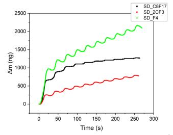
Fig. 6 Mass changes of the gold-quartz electrode ( $S = 5 \text{ mm}^2$ ) measured by EQCM during the electrochemical grafting (10 cycles) of 1 mM solutions of DS\_C8F17, DS\_2(CF3) and DS\_F4 salts.
