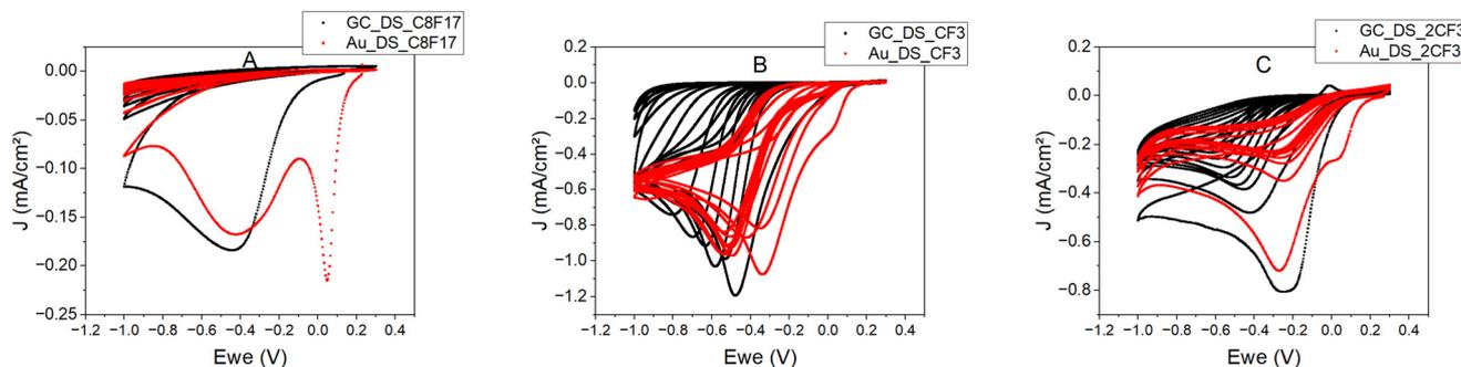
Fig. 4 Cyclic voltammograms recorded at a sweep rate of  $100 \text{ mV s}^{-1}$  on GC (black) and gold (red) electrodes in  $1 \text{ mM}$  solutions of **DS\_C8F17** (A), **DS\_CF3** (B), and **DS\_2(CF3)** (C) salts. The salts were dissolved in a  $n\text{-NBu}_4\text{PF}_6/\text{ACN}$  electrolyte. All potentials are reported versus an  $\text{Ag}/\text{Ag}^+$  reference electrode, with a platinum gauze as counter electrode.
