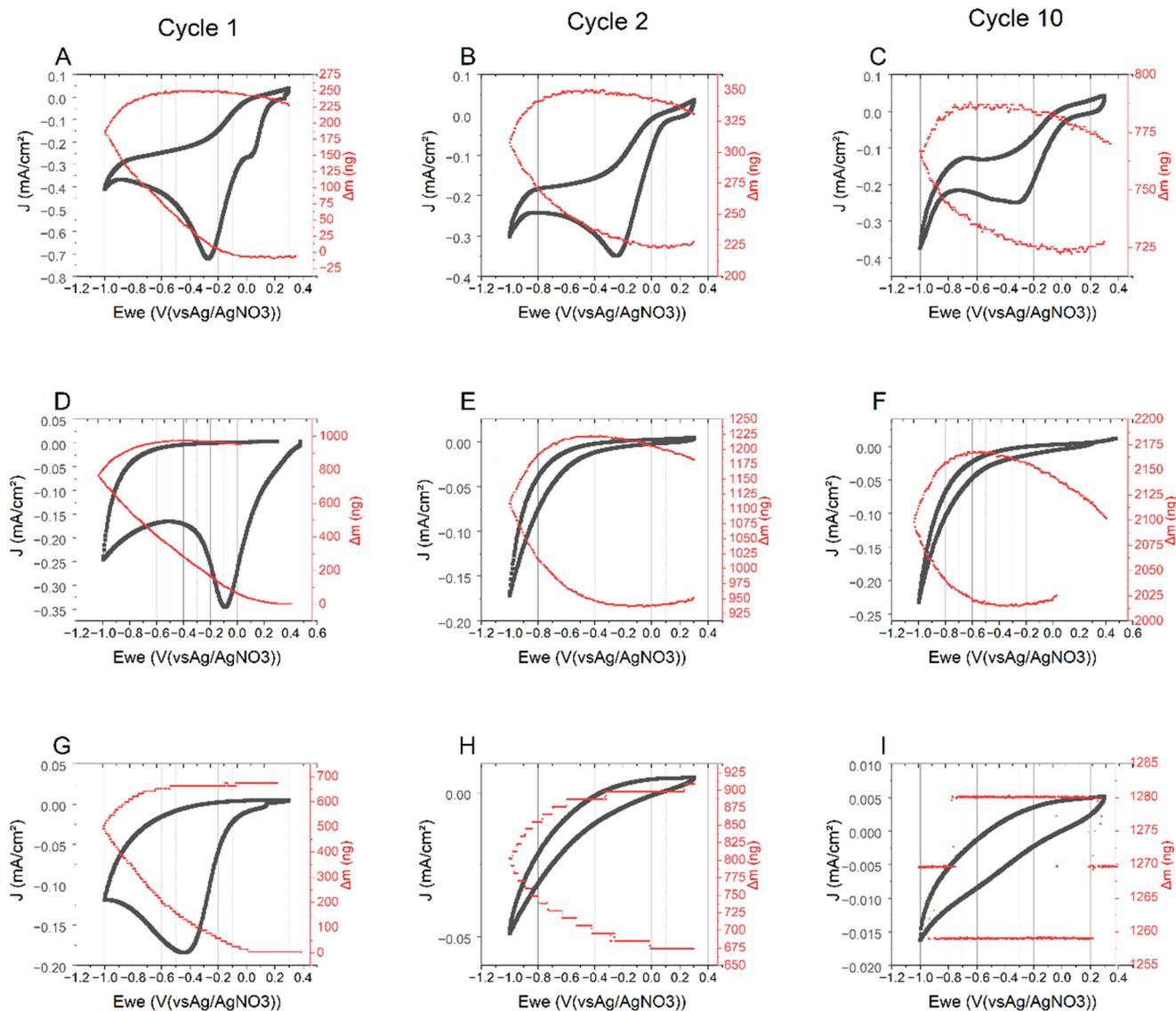
Fig. 7 Mass change and CV of the gold-quartz electrode for cycle 1, 2 and 10 for DS<sub>2</sub>(CF<sub>3</sub>) (A–C), DS<sub>F4</sub> (D–F) and DS<sub>C8F17</sub> (G–I). All curves were recorded in acetonitrile (AN) with 0.1 M nBu<sub>4</sub>PF<sub>6</sub> at a scan rate of 50 mV s<sup>-1</sup> over 10 cycles between [-1 V; Eoc] versus Ag/Ag<sup>+</sup>.
