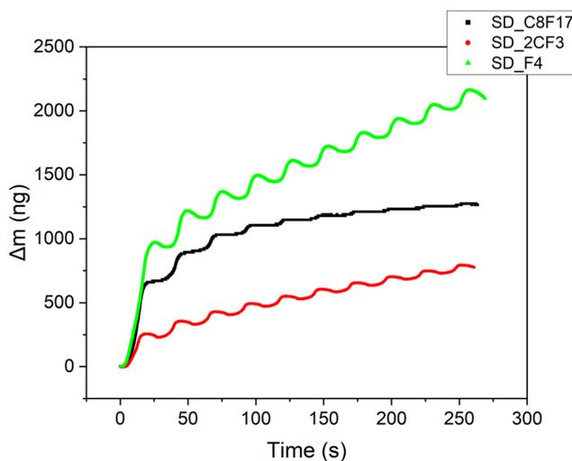
Fig. 6 Mass changes of the gold-quartz electrode ( $S = 5 \text{ mm}^2$ ) measured by EQCM during the electrochemical grafting (10 cycles) of  $1 \text{ mM}$  solutions of DS\_C8F17, DS\_2(CF3) and DS\_F4 salts.
