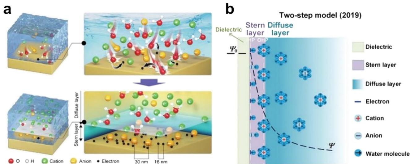
Fig. 3 The 'two-step' EDL model at the dielectric-liquid interface proposed in 2019. (a) The mechanism of electron transfer and ion adsorption is considered in the 'two-step' formation process.<sup>64</sup> (b) The 'two-step' model of EDL structure and charge composition.<sup>65</sup>
