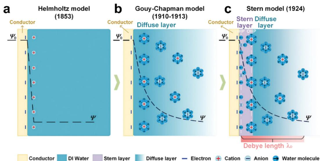
Fig. 2 The development history of the EDL model.<sup>57</sup> (a) The Helmholtz model. (b) The Gouy–Chapman model. (c) The Stern model.
