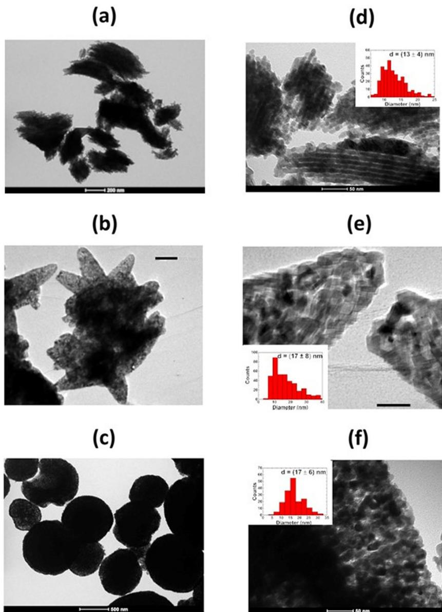
Fig. 1 Typical TEM images of (a and d) O-MnO<sub>2</sub>, (b and e) D-MnO<sub>2</sub> and (c and f) D-Mn<sub>2</sub>O<sub>3</sub> samples at distinct magnifications and the respective histograms of their size distribution.
