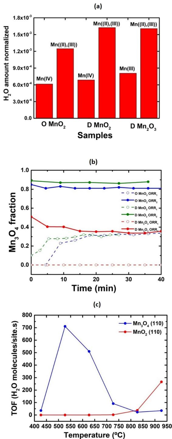
Fig. 4 (a) H<sub>2</sub>O amount normalized by the surface area before (left) and after (right) reduction treatment for each sample. (b) Time evolution of the Mn<sub>3</sub>O<sub>4</sub> fraction during the ORR before (open circles) and after (solid circles) reduction treatment. (c) ORR turnover frequency as a function of temperature for  $\beta$ -MnO<sub>2</sub> (110) and Mn<sub>3</sub>O<sub>4</sub> (110) surfaces. Obtained from KMC simulations.
