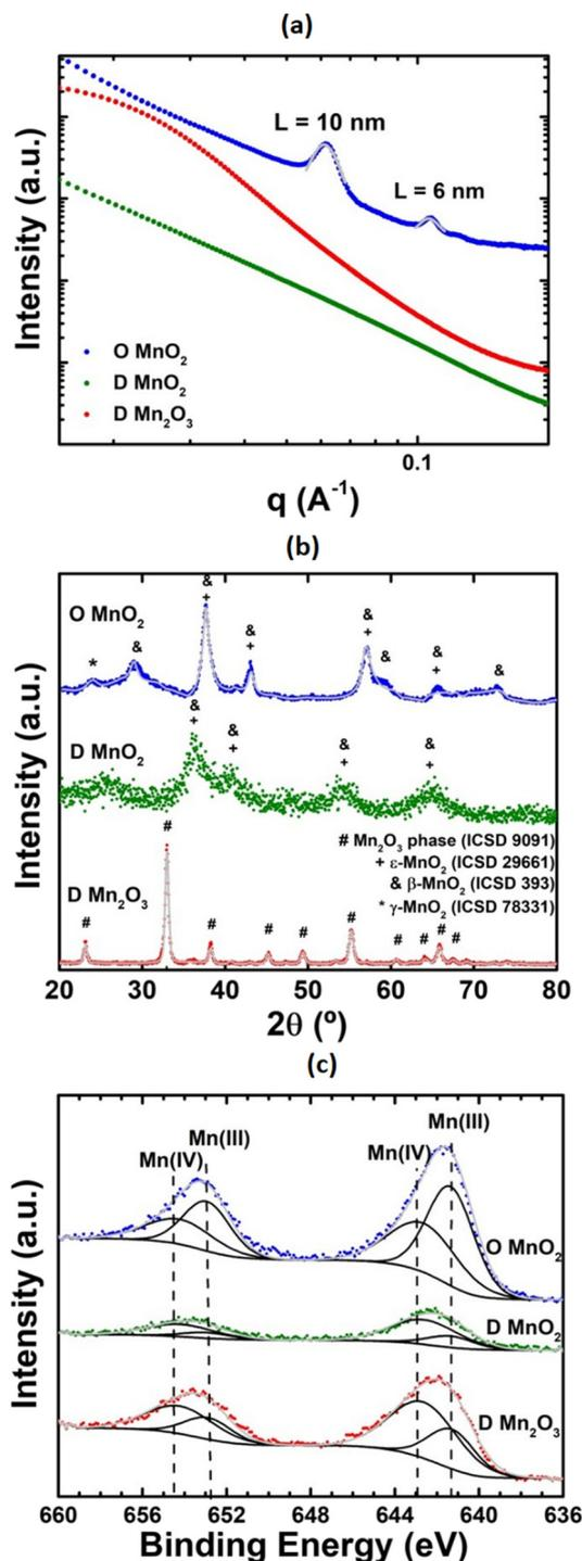
Fig. 2 (a) SAXS patterns, (b) XRD patterns with the corresponding Rietveld refinement result, and (c) Mn 2p XPS spectra of O-MnO<sub>2</sub>, D-MnO<sub>2</sub>, and D-Mn<sub>2</sub>O<sub>3</sub> samples.
