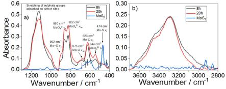
Fig. 3 a) FTIR absorption spectra, in the 1300-400 cm<sup>-1</sup> range, of MoS<sub>2</sub> (blue line) and Na<sub>2</sub>MoO<sub>4</sub> (20 h) (red line) and Na<sub>2</sub>MoO<sub>4</sub> (8 h) (black line) exfoliated products. The weak and narrow bands detected at lower wavelengths are indicated by a black segment. b) FTIR absorption spectra, in the 3750-2800 cm<sup>-1</sup> range.
