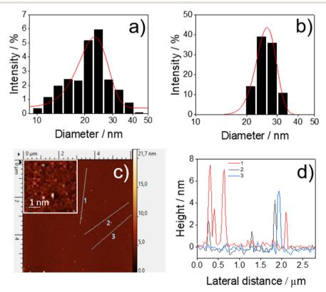
Fig. 5 Dynamic light scattering of the exfoliated samples after a) 8 h and b) 20 h thermally assisted exfoliation. The red line is a guide for the eyes. c) AFM image of the Na<sub>2</sub>MoO<sub>4</sub> (8 h) nanoparticles. The inset shows a magnified view of the NPs. d) Dimensional profiles of the nanoparticles; the curves correspond to the lines 1, 2 and 3 in c).
