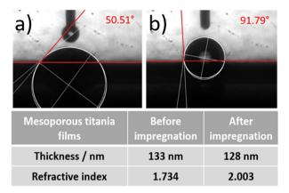
Fig. 9 Contact angles of mesoporous titania films, before (a) and after impregnation with Na<sub>2</sub>MoO<sub>4</sub> (8 h) NPs (b). The table lists the thickness and refractive index before and after impregnation with the nanoparticles
