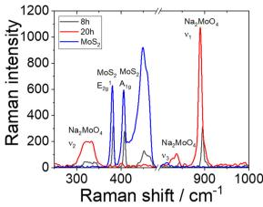
Fig. 4 Raman spectra of MoS<sub>2</sub> (blue line) and reaction products Na<sub>2</sub>MoO<sub>4</sub> (8 h) (black line) and Na<sub>2</sub>MoO<sub>4</sub> (20 h) (red line) at 200 °C. Laser excitation wavelength:  $\lambda = 785$  nm.
