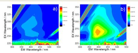
Fig. 7 Fluorescence map (x-emission, y-excitation, z-intensity on the false colour scale) of Na<sub>2</sub>MoO<sub>4</sub> (8 h) (a) and Na<sub>2</sub>MoO<sub>4</sub> (20 h) (b) treated samples.
