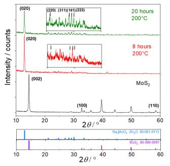
Fig. 2 XRD patterns of precursor MoS<sub>2</sub> (black line) and samples obtained after thermally assisted exfoliation for 8 (red line) and 20 hours (green line) at 200 °C, respectively. The inset shows a magnified view of the corresponding pattern. The bottom panel shows the standard XRD patterns of sodium molybdate dihydrate (blue) (JCPDS card 00-001-0113) and crystalline hexagonal MoS2 (violet) (JCPDS card 00-006-0097).
