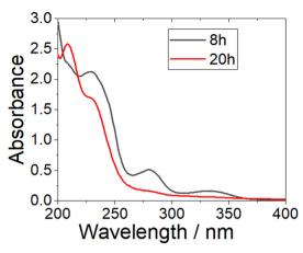
Fig. 6 UV-vis absorption spectra of Na<sub>2</sub>MoO<sub>4</sub> (8 h) (black line) and Na<sub>2</sub>MoO<sub>4</sub> (20 h) (red line) agueous dispersions (concentration of 3 mg  $mL^{-1}$ ).
