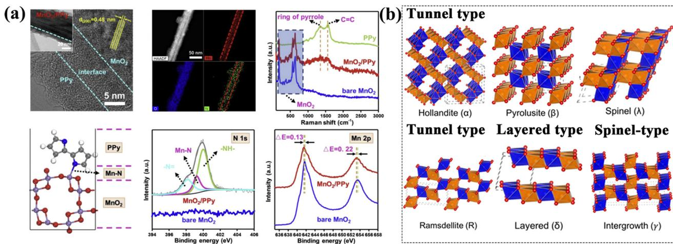
Fig. 3 (a) Characterizations of  $\text{MnO}_2$ /polypyrrole electrode for ZIBs, including TEM (inset), HRTEM, Raman, and XPS. Reproduced with permission from ref. 72. Copyright 2020. Elsevier. (b) Different  $\text{MnO}_2$  polymorphs. Reproduced with permission from ref. 73. Copyright 2018, American Chemical Society.
