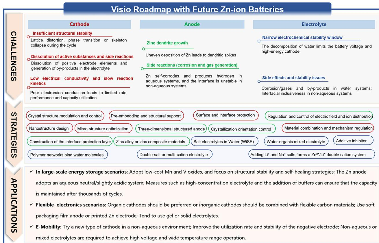
Fig. 13 The visio roadmap with future Zn-ion batteries.
