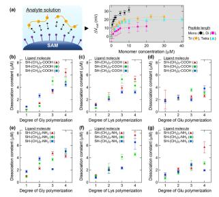
Fig. 4 Analysis of the interactions per amino acid unit. (a) Schematic of AAIs and an example of the electrical response at the monoamino acid scale. (b-g) Dissociation constants depending on the chain lengths of the (b and e) Gly, (c and f) Lys, and (d and g) Glu peptides using the SAMs comprising (b-d) carboxy or (e-g) amino groups. Error bars represent the standard deviation obtained from the Hill-Waud fitting.
