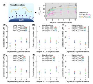
Fig. 3 Analysis of the interactions between peptides and accumulated charged residues. (a) Schematic of AAIs and an example of an electrical response at the peptide scale. (b-g) Dissociation constants depending on the chain lengths of (b and e) Gly, (c and f) Lys, and (d and g) Glu peptides using the SAMs comprising (b-d) carboxy or (e-g) amino groups. Error bars represent the standard deviation obtained from the Hill-Waud fitting
