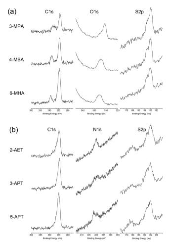
Fig. 2 C 1s, S 2p, O 1s, and N 1s X-ray photoelectron spectra of the Au surfaces modified with self-assembled monolayers comprising (a) mercaptocarboxylic acids or (b) aminoalkanethiols.
