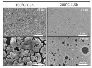
Fig. 7 SEM observations (surfaces) of annealed ZnO: Ga samples after reaction/conversion in a CH<sub>3</sub>OH/H<sub>2</sub>O mixture (3:1) at different temperatures (100 °C and 200 °C) for 1.5 h.
