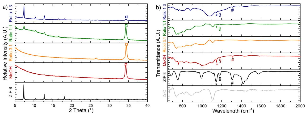
**Fig. 3** a) XRD patterns of ZnO:Ga samples reacted/converted at 100 °C for 1.5 h in different CH<sub>3</sub>OH/H<sub>2</sub>O mixtures (ratios 1:3, 1:1 and 3:1), compared with the theoretical pattern of ZIF-8. (□) indicates ZnO diffraction peak; b) corresponding FTIR spectra, with (\*) *H*<sub>ring</sub> wag, (§) ring breathing (C-N symmetric stretch), and (#) *H*<sub>methyl</sub> scissor, characteristic absorption bands of ZIF-8.
