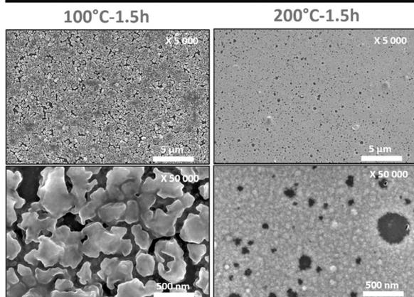
Fig. 7 SEM observations (surfaces) of annealed ZnO:Ga samples after reaction/conversion in a CH<sub>3</sub>OH/H<sub>2</sub>O mixture (3:1) at different temperatures (100 °C and 200 °C) for 1.5 h.
