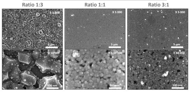
Fig. 4 SEM observations (surfaces) of ZnO: Ga samples after reaction/conversion at 100  $^{\circ}$ C for 1.5 h in CH<sub>3</sub>OH/H<sub>2</sub>O solvent mixtures with different ratios (1:3; 1:1 and 3:1).
