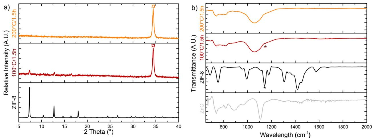
**Fig. 6** a) XRD patterns of annealed ZnO:Ga samples reacted/converted in a CH<sub>3</sub>OH/H<sub>2</sub>O mixture (3:1) at 100 °C or 200 °C for 1.5 h, compared with the theoretical pattern of ZIF-8. (⊠) indicates ZnO diffraction peak; b) corresponding FTIR spectra, with (#)  $H_{ring}$  wag vibrational band, characteristic of ZIF-8.
