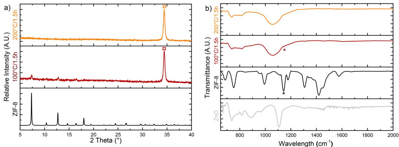
**Fig. 6** a) XRD patterns of annealed ZnO:Ga samples reacted/converted in a CH<sub>3</sub>OH/H<sub>2</sub>O mixture (3:1) at 100 °C or 200 °C for 1.5 h, compared with the theoretical pattern of ZIF-8. (⊠) indicates ZnO diffraction peak; b) corresponding FTIR spectra, with (#) *H*<sub>ring</sub> wag vibrational band, characteristic of ZIF-8.
