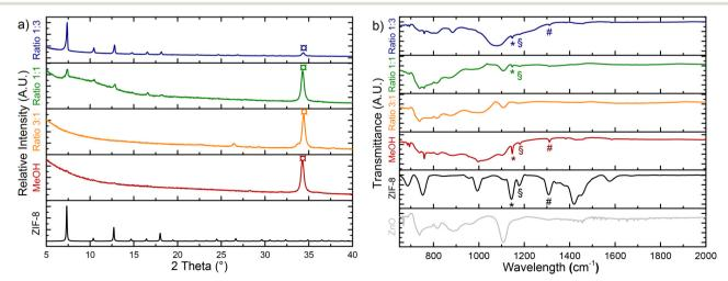
Fig. 3 a) XRD patterns of ZnO: Ga samples reacted/converted at 100 °C for 1.5 h in different CH<sub>3</sub>OH/H<sub>2</sub>O mixtures (ratios 1:3, 1:1 and 3:1), compared with the theoretical pattern of ZIF-8. ( $\mathfrak{X}$ ) indicates ZnO diffraction peak; b) corresponding FTIR spectra, with (\*)  $H_{\text{ring}}$  wag, (§) ring breathing (C–N symmetric stretch), and (#)  $H_{\text{methyl}}$  scissor, characteristic absorption bands of ZIF-8.
