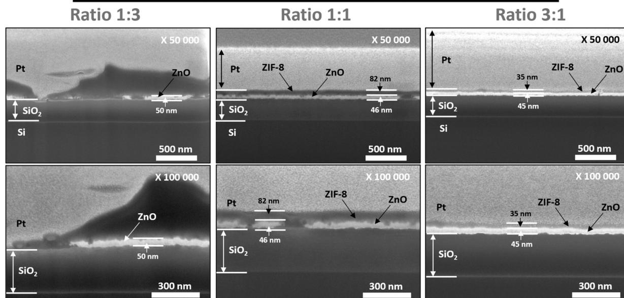
Fig. 5 SEM observations (cross-sections) of ZnO:Ga samples after reaction/conversion at 100 °C for 1.5 h in CH<sub>3</sub>OH/H<sub>2</sub>O solvent mixtures with different ratios (1:3; 1:1 and 3:1).
