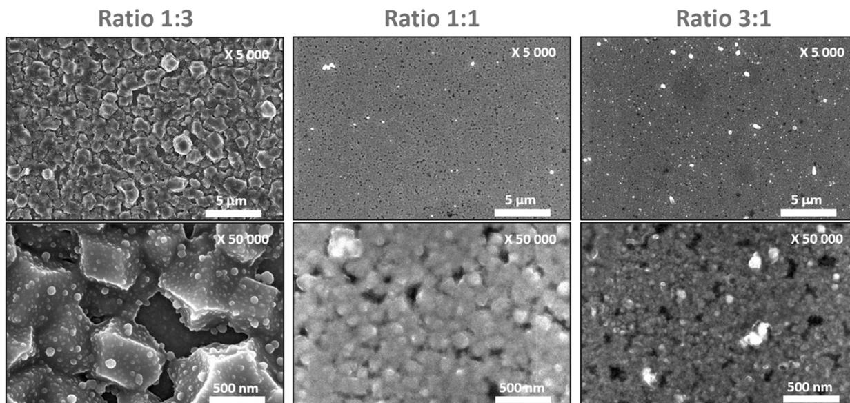
Fig. 4 SEM observations (surfaces) of ZnO:Ga samples after reaction/conversion at 100 °C for 1.5 h in CH<sub>3</sub>OH/H<sub>2</sub>O solvent mixtures with different ratios (1 : 3; 1 : 1 and 3 : 1).
