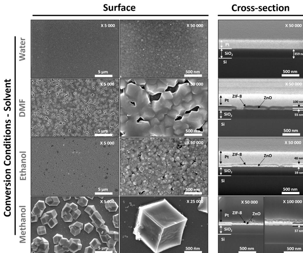
Fig. 2 SEM observations (surfaces and cross-sections) of ZnO:Ga samples after reaction/conversion at 100 °C for 12 h in various solvents (water, DMF, ethanol or methanol).
