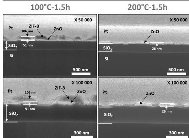
Fig. 8 SEM observations (cross-sections) of annealed ZnO:Ga samples after reaction/conversion in a CH<sub>3</sub>OH/H<sub>2</sub>O mixture (3:1) at different reaction temperatures (100 °C and 200 °C) for 1.5 h.
