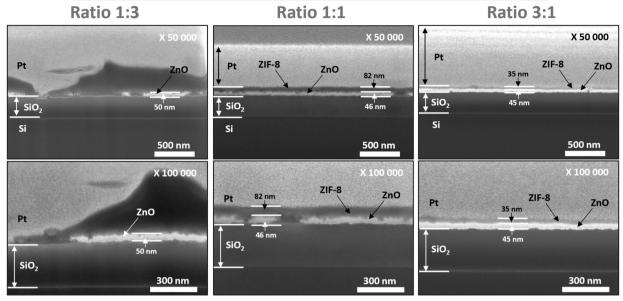
Fig. 5 SEM observations (cross-sections) of ZnO: Ga samples after reaction/conversion at 100 °C for 1.5 h in CH₃OH/H₂O solvent mixtures with different ratios (1:3; 1:1 and 3:1).
