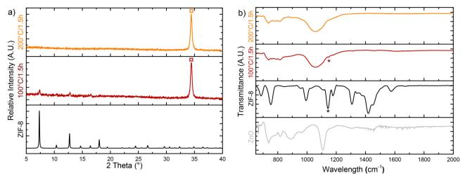
Fig. 6 a) XRD patterns of annealed ZnO: Ga samples reacted/converted in a CH $_3$ OH/H $_2$ O mixture (3:1) at 100 °C or 200 °C for 1.5 h, compared with the theoretical pattern of ZIF-8. ( $\not a$ ) indicates ZnO diffraction peak; b) corresponding FTIR spectra, with (#)  $H_{ring}$  wag vibrational band, characteristic of ZIF-8.
