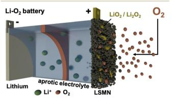
**Fig. 1** Scheme of Li–O $_2$  battery with La $_{0.7}$ Sr $_{0.3}$ Mn $_{1-x}$ Ni $_x$ O $_3$  double perovskite catalyst (LSMN) in the cathode. Red, green and yellow spheres correspond to lithium ions, oxygen, and superoxide/peroxide compounds, respectively.
