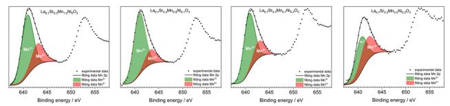
Fig. 7 Mn 2p XPS spectra for pristine  $La_{0.7}Sr_{0.3}Mn_1Ni_0O_3$ ,  $La_{0.7}Sr_{0.3}Mn_{0.9}Ni_{0.1}O_3$ ,  $La_{0.7}Sr_{0.3}Mn_{0.7}Ni_{0.3}O_3$ , and  $La_{0.7}Sr_{0.3}Mn_{0.5}Ni_{0.5}O_3$  catalyst demonstrating population of  $Mn^{3+}$  on the oxide surface depending on the Ni substitution ratio. The molar ratios of  $Mn^{3+}/Mn^{4+}$  determined from fitting analysis are listed in ESI.†
