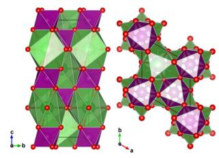
Fig. 2 Crystallographic structure of the AA'BB'O<sub>3</sub> double perovskite of La<sub>0.7</sub>Sr<sub>0.3</sub>Mn<sub>1</sub>Ni<sub>0</sub>O<sub>3</sub> compound having a 167  $R\bar{3}c$  symmetry. The unit cell dimensions are a=5.50300 Å, b=5.50300 Å, c=13.4241 Å and cell volume of 349.916086 Å<sup>3</sup>.
