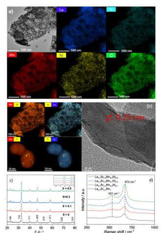
Fig. 3 TEM and corresponding EDS elemental mapping for La, Sr, Mn Ni, O and superimposed MnNi and NiLa (a and b), (c) ex situ XRD patterns and (d) ex situ Raman spectra of  $La_{0.7}Sr_{0.3}Mn_{1-x}Ni_xO_3$  (x = 0, 0.1, 0.3, 0.5) pristine catalyst.
