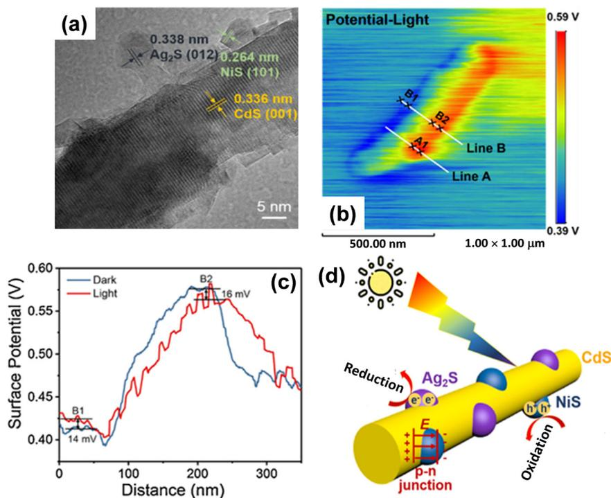
Fig. 4 (a) HRTEM image of CdS/Ag<sub>2</sub>S/NiS. (b) KPFM image of CdS/Ag<sub>2</sub>S/NiS under light irradiation of 420 nm. (c) Surface potential profiles under 420 nm light irradiation. (d) Pictorial representation of electron and hole migration process in CdS/Ag<sub>2</sub>S/NiS under illumination. Reproduced from ref. 44 with permission from [Elsevier], copyright [2021].
