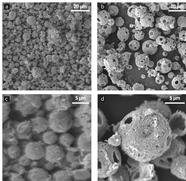
**Fig. 2** SEM images of mesoporous  $V_2O_5$  microspheres.  $V_2O_5$  microspheres synthesized from emulsions containing different ratios of BCP to hexadecane. a and c) 100 : 0; b and d) 70 : 30. While porosity on the 10 nm scale is present in all samples, the 70 : 30 spheres exhibit micrometer-sized pores resulting from the addition of hexadecane.
