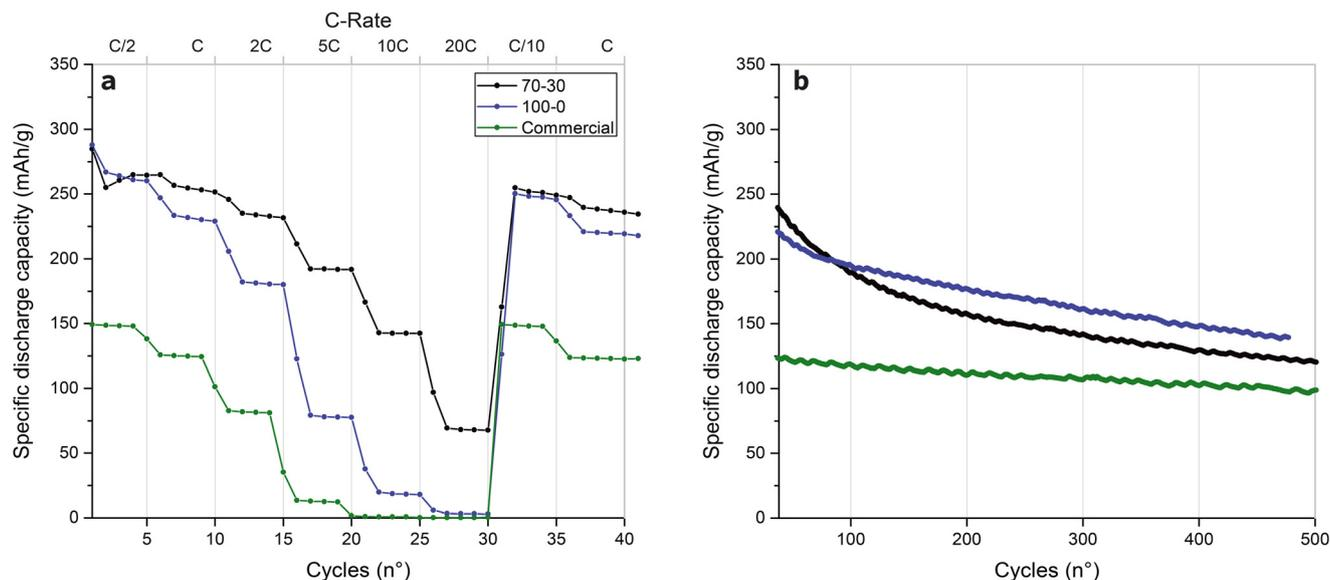
**Fig. 5** Electrochemical performance of  $V_2O_5$  electrodes with different microporosities. Rate capability (a) and calendar tests (b) of  $V_2O_5$  microsphere electrodes prepared from templates made with different BCP : hexadecane ratios (70 : 30 and 100 : 0) cycled using LiTFSI in tetraglyme as electrolyte, compared to an unstructured, commercial  $V_2O_5$ .
