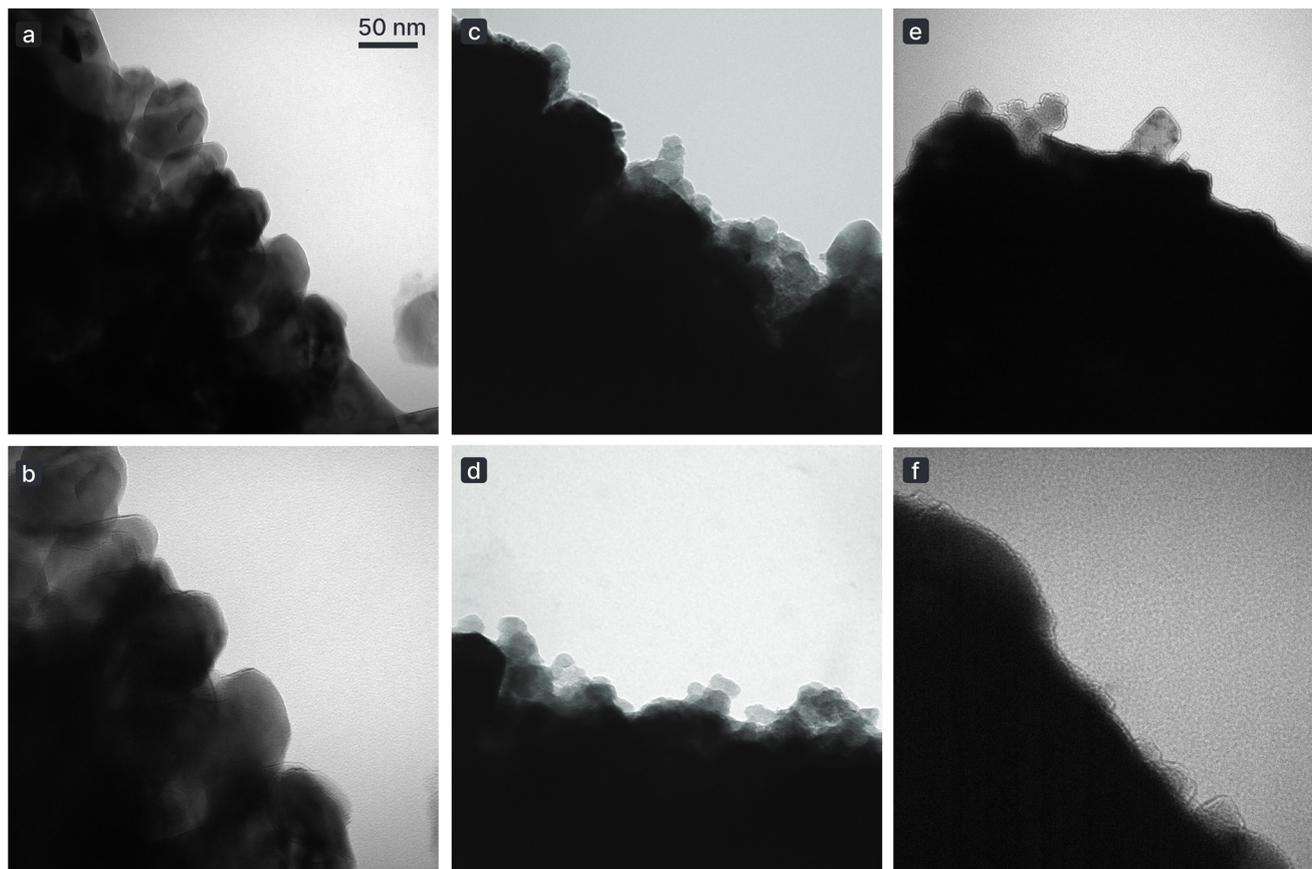
**Fig. 4** Transmission electron microscopy images of  $V_2O_5$  surfaces before and after electrochemical cycling. (a and b) Pristine  $V_2O_5$  70 : 30 surface with well-defined crystalline structures. (c and d) Similar  $V_2O_5$  surface after 75 cycles with  $LiPF_6$  in EC : DMC electrolyte, showing non-uniform SEI layer formation. (e and f) When LiTFSI in tetraglyme is used as electrolyte, only a few lumpy SEI aggregates separated by a very thin, uniform SEI layer are observed.
