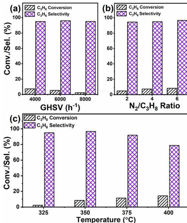
Fig. 3 Effect of GHSV (a), effect of N<sub>2</sub>/C<sub>3</sub>H<sub>8</sub> (b) and effect of temperature on the conversion of C<sub>3</sub>H<sub>8</sub> and selectivity for C<sub>3</sub>H<sub>6</sub> during propane dehydrogenation (c). Reaction conditions: Wt of catalyst–0.25 g (pelletised); reaction temperature, 350 °C (for a and b); GHSV–4000 h<sup>-1</sup> (for b and c).
