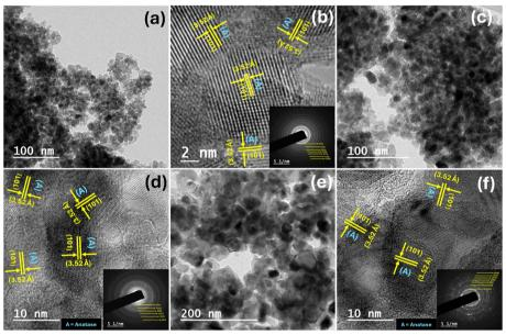
Fig. 2 TEM and HRTEM with the SAED patterns of (a and b) TiO<sub>2</sub>, (c and d) fresh and (e and f) spent Cu-TiO<sub>2</sub> catalysts.
