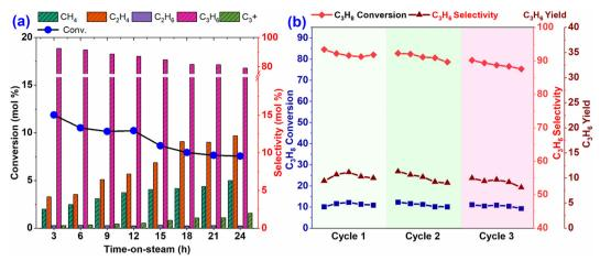
Fig. 4 (a) TOS and (b) regeneration cycles over the Cu-TiO<sub>2</sub> catalyst in terms of propane conversion, propylene selectivity, and propylene yield. Reaction conditions: Wt of catalyst-0.25 g (pelletized); reaction temperature, 375 °C; GHSV-4000 h<sup>-1</sup>.
