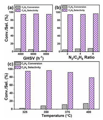
Fig. 3 Effect of GHSV (a), effect of N2/C3H8 (b) and effect of temperature on the conversion of C<sub>3</sub>H<sub>8</sub> and selectivity for C<sub>3</sub>H<sub>6</sub> during propane dehydrogenation (c). Reaction conditions: Wt of catalyst-0.25 g (pelletised); reaction temperature, 350 °C (for a and b); GHSV-4000  $h^{-1}$  (for b and c).
