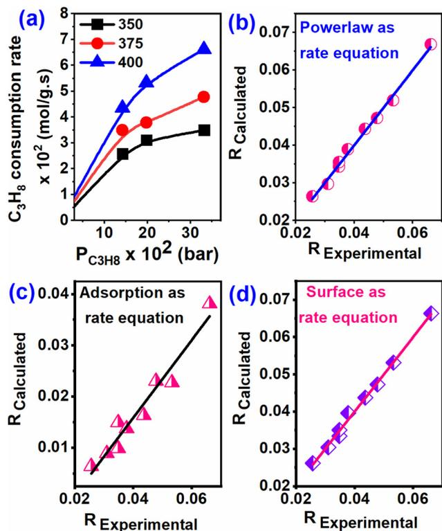
Fig. 5 (a) Dependence of the rates of C<sub>3</sub>H<sub>8</sub> consumption over Cu-TiO<sub>2</sub> measured at 350, 375, and 400 °C on the C<sub>3</sub>H<sub>8</sub> partial pressure. (b–d) Plot of R<sub>Calculated</sub> vs. R<sub>Observed</sub> of the data taken between 350 and 400 °C.
