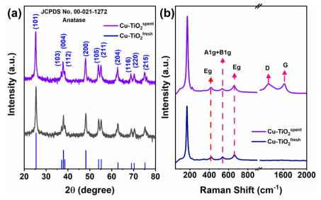
Fig. 1 (a) XRD and (b) Raman spectra for fresh and spent Cu-TiO<sub>2</sub> catalysts.
