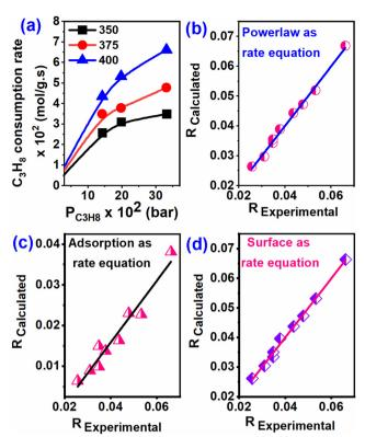
Fig. 5 (a) Dependence of the rates of C<sub>3</sub>H<sub>8</sub> consumption over Cu-TiO<sub>2</sub> measured at 350, 375, and 400 °C on the C<sub>3</sub>H<sub>8</sub> partial pressure. (b-d) Plot of Rcalculated vs. Robserved of the data taken between 350 and 400 °C.
