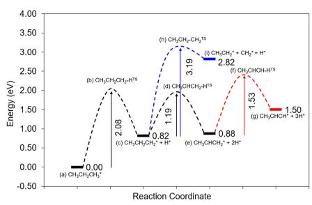
Fig. 6 Energy diagram from propane dehydrogenation to propylene (black colour), propylene dehydrogenation (red colour) and C-C bond cleavage of the CH<sub>3</sub>CH<sub>2</sub>CH<sub>2</sub> intermediate (blue colour).
