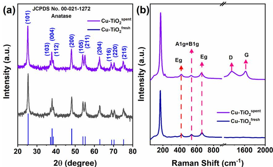
Fig. 1 (a) XRD and (b) Raman spectra for fresh and spent Cu-TiO<sub>2</sub> catalysts.
