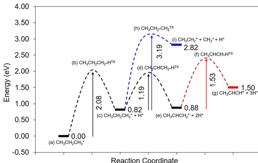
Fig. 6 Energy diagram from propane dehydrogenation to propylene (black colour), propylene dehydrogenation (red colour) and C–C bond cleavage of the  $\text{CH}_3\text{CH}_2\text{CH}_2$  intermediate (blue colour).
