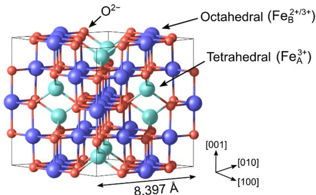
**Fig. 1** The bulk structure of  $\text{Fe}_3\text{O}_4$  at low temperature is based on an fcc arrangement of  $\text{O}^{2-}$  cations (red), where  $\text{Fe}^{3+}$  cations occupy tetrahedral sites ( $\text{Fe}_A$ , cyan), and a 1:1 mixture of  $\text{Fe}^{2+}$  and  $\text{Fe}^{3+}$  cations resides in octahedral sites ( $\text{Fe}_B$ , dark blue). The experimental lattice parameter at room temperature is 8.397 Å.
