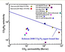
Fig. 10 CO<sub>2</sub>/N<sub>2</sub> separation performances of the MPSf-ZIF-90@CNTs, MPSf-ZIF-90@c-CNTs and other MMMs in Robeson's upper bound (2008) plot.
