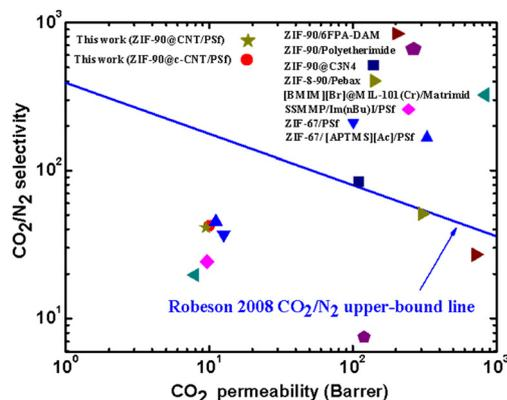
Fig. 10 CO<sub>2</sub>/N<sub>2</sub> separation performances of theMPSf-ZIF-90@CNTs, MPSf-ZIF-90@c-CNTs and other MMMs in Robeson's upper bound (2008) plot.
