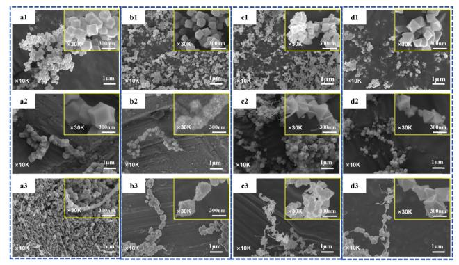
Fig. 5 SEM images of (a1-a3) ZIF-8, ZIF-8@CNTs and ZIF-8@c-CNTs, (b1-b3) MOF-801, MOF-801, MOF-801@CNTs and MOF-801@c-CNTs, (c1-c3) UiO-66, UiO-66@CNTs and UiO-66@c-CNTs, and (d1-d3) UiO-66-NH2, UiO-66-NH2@CNTs and UiO-66-NH2@c-CNTs.
