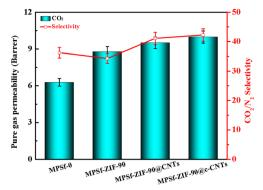
Fig. 9 Pure CO<sub>2</sub> permeability and ideal CO<sub>2</sub>/N<sub>2</sub> selectivity of MPSf-0, MPSf-ZIF-90, MPSf-ZIF-90@CNTs and MPSf-ZIF-90@c-CNTs.
