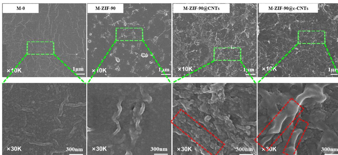
Fig. 6 SEM images of M-0, M-ZIF-90, M-ZIF-90@CNTs and M-ZIF-90@c-CNTs.
