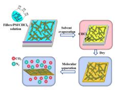
**Scheme 3** Schematic illustration for the process of preparing MOF@CNTs-based gas separation membranes for molecular separation.
