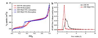
Fig. 3 (a)  $N_2$  adsorption–desorption isotherms at 77 K and (b) pore size distribution data of the as-synthesized ZIF-90 and ZIF-90@CNTs-0.05.
