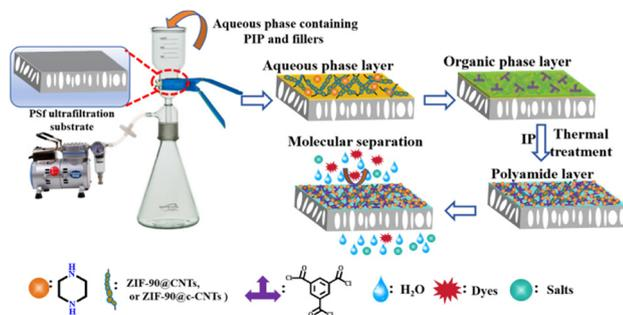
**Scheme 2** Schematic illustration for the process of preparing MOF@CNTs-based nanofiltration membranes for molecular separation.
