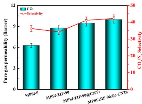
Fig. 9 Pure CO<sub>2</sub> permeability and ideal CO<sub>2</sub>/N<sub>2</sub> selectivity of MPSf-0, MPSf-ZIF-90, MPSf-ZIF-90@CNTs and MPSf-ZIF-90@c-CNTs.
