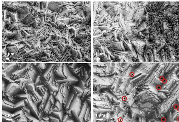
**Fig. 2** SEM images of ZE coated with PT 1 (top) and PT 2 (bottom) after alkaline cleaning (left) and acidic cleaning (right). Formed pores have been highlighted by red circles.
