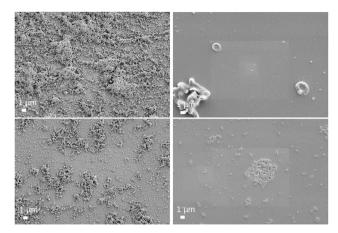
Fig. 12 SEM images of model surfaces coated with PT 1 on zinc (top left), aluminium (top right) or magnesium (bottom). Magnesium center of the sample (bottom left) and area closer to the edges (bottom right).
