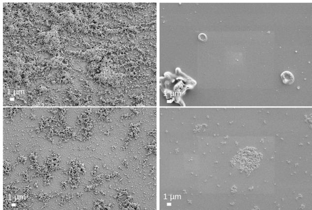
**Fig. 12** SEM images of model surfaces coated with PT 1 on zinc (top left), aluminium (top right) or magnesium (bottom). Magnesium – center of the sample (bottom left) and area closer to the edges (bottom right).
