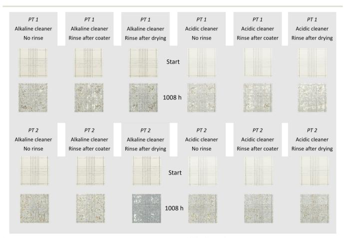
Fig. 8 Visual images of coated samples before and after water storage test for 1008 h (6 weeks) for ZM substrate.
