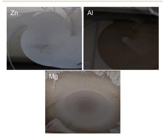
Fig. 11 Visual images of model surfaces (45 mm  $\times$  45 mm) of zinc, aluminium or magnesium, coated with PT 1 by spin-coating, after drying.
