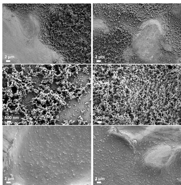
Fig. 4 SEM images of ZM coated with PT 1 (top and middle; middle with higher magnification) and PT 2 (bottom) after alkaline cleaning (left) and acidic cleaning (right).
