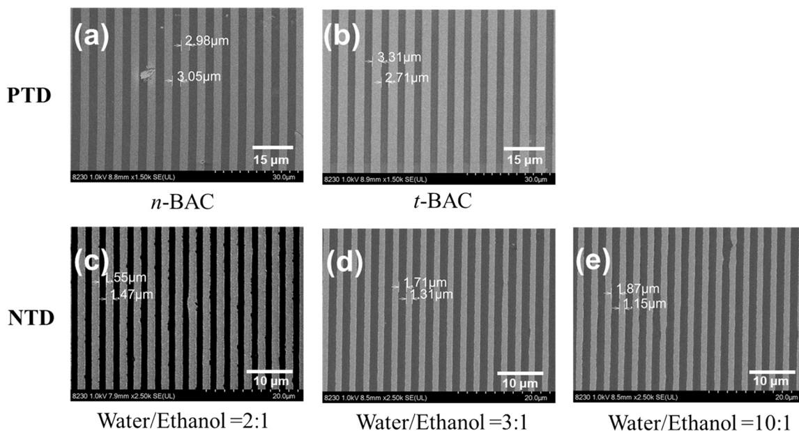
**Fig. 3** The SEM images of ADTPS resist patterns developed in (a) *n*-BAC (3  $\mu\text{m}$ ), (b) *t*-BAC (3  $\mu\text{m}$ ), (c) water/ethanol (2 : 1) mixture (1.5  $\mu\text{m}$ ), (d) water/ethanol (3 : 1) mixture (1.5  $\mu\text{m}$ ), and (e) water/ethanol (10 : 1) mixture (1.5  $\mu\text{m}$ ) by DUV (254 nm) exposure at  $25 \text{ mJ cm}^{-2}$ .
