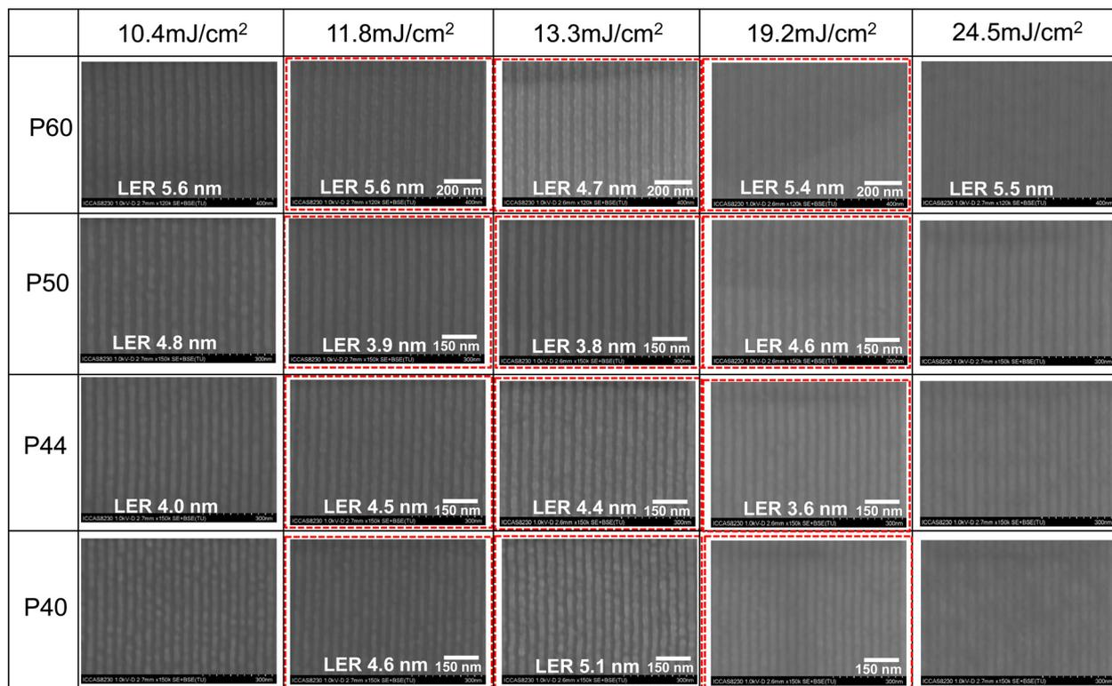
Fig. 6 The SEM images of the 30, 25, 22 and 20 nm HP line patterns of the ADTPS resist at different exposure doses (thickness: 30 nm; developer: water/ethanol = 2/1).
