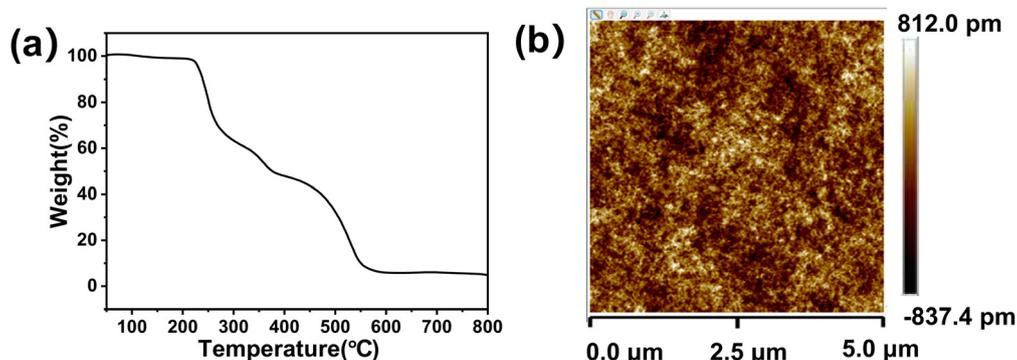
Fig. 2 (a) TGA curve of ADTPS; (b) two-dimensional AFM image of the ADTPS film.
