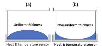
Fig. 7 Molten salt in DSC container. (a) Appropriate contact with uniform thickness: (b) inappropriate contact with non-uniform thickness
