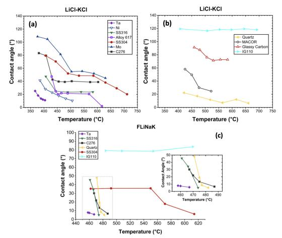
Fig. 4 LiCI-KCI and FLiNaK contact angle change trend with temperature: (a) LiCI-KCI on metal substrates; (b) LiCI-KCI on non-metal substrates; (c) FLiNaK on metal and non-metal substrates
