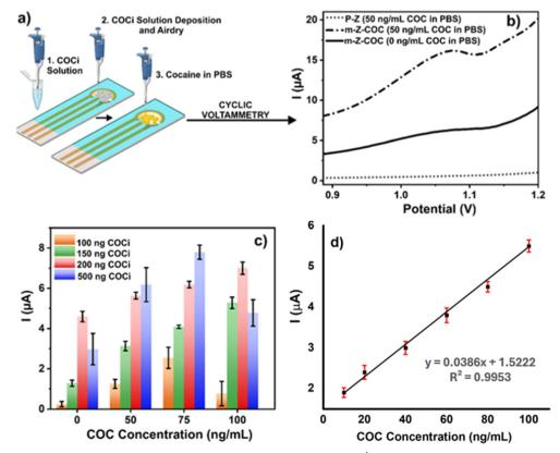
Fig. 3 a) Schematic of electrode modification. b) SWV detection of cocaine (50 ng mL<sup>-1</sup>) using P-Z and m-Z-COC in PBS. c) Cocaine detection using different amounts of COCi to modify the electrode, and d) calibration curve for cocaine detection in PBS using m-Z-COC (COCi 150 ng).
