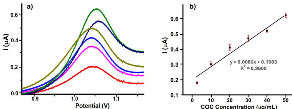
Fig. 1 a) SWV signals of different amounts of cocaine and b) calibration curve for cocaine detection in PBS using P-Z.
