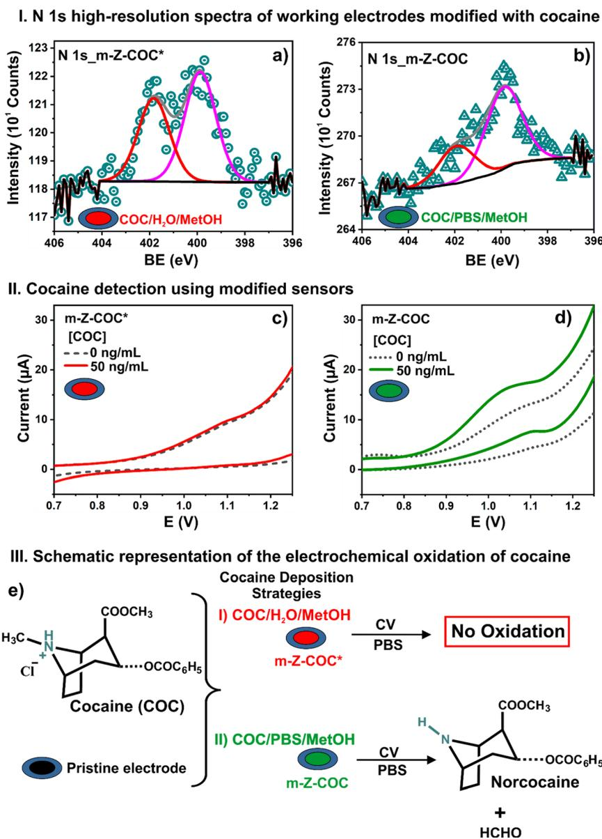
Fig. 2 N 1s high-resolution spectra of a) m-Z-COC\* and b) m-Z-COC. Cocaine detection using c) m-Z-COC\* and d) m-Z-COC electrodes employing CV. e) Schematic representation of the electrochemical oxidation mechanism for cocaine.
