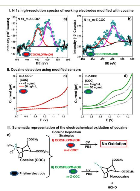
Fig. 2 N 1s high-resolution spectra of a) m-Z-COC\* and b) m-Z-COC. Cocaine detection using c) m-Z-COC\* and d) m-Z-COC electrodes employing CV. e) Schematic representation of the electrochemical oxidation mechanism for cocaine.
