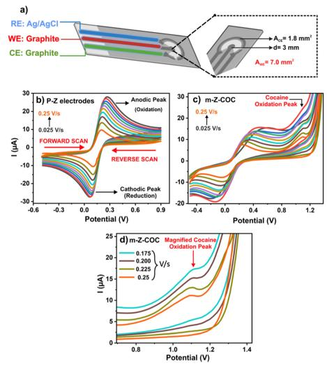
Fig. 5 (a) Configuration of a Zensor electrode. (b) CV response of a P-Z with different scan rates. (c) CV response of m-Z-COC with different scan rates. (d) Magnified cocaine peak in m-Z-COC scans.
