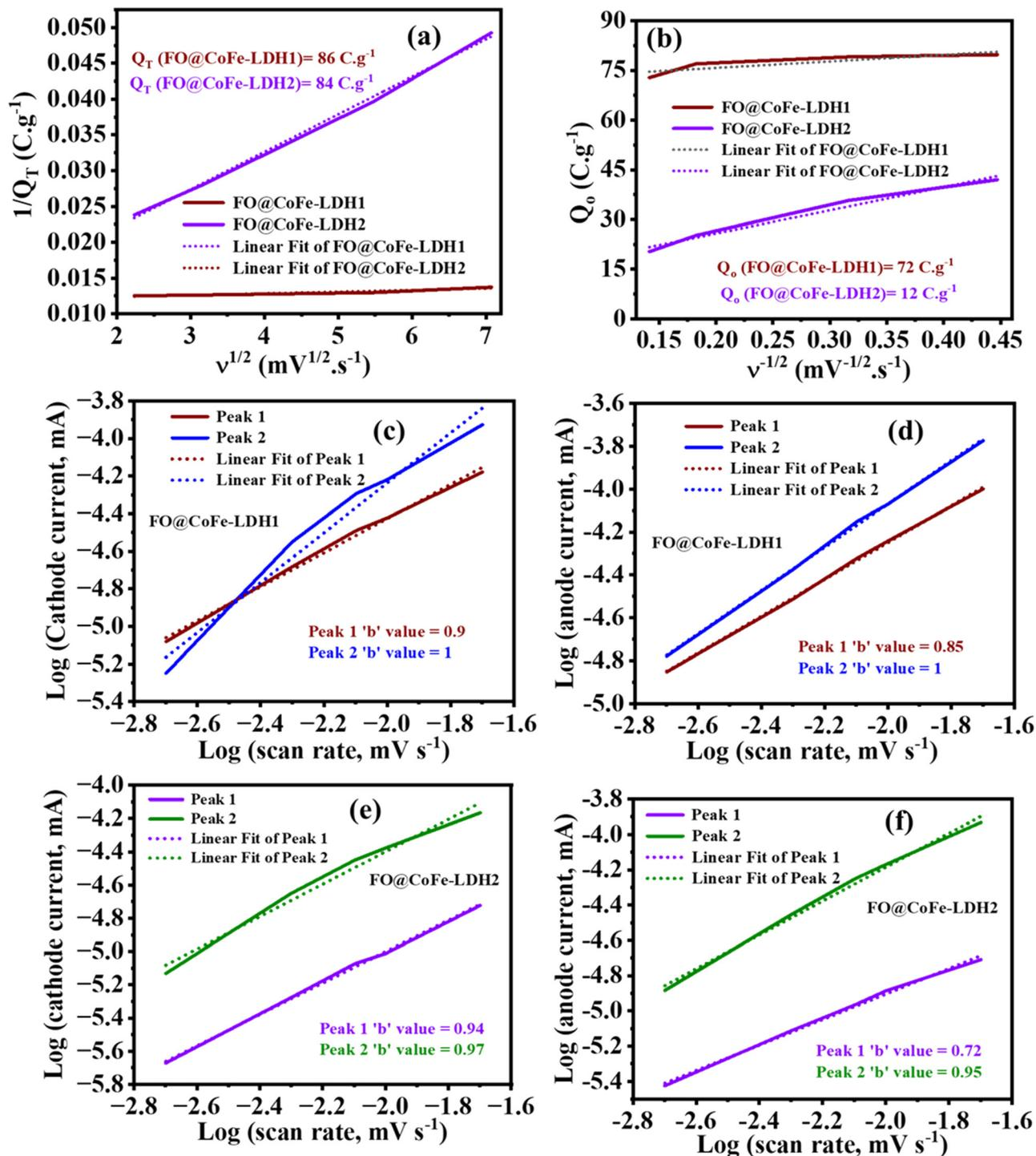
Fig. 8 (a and b) Trasatti methods for FO@CoFe-LDH1 and FO@CoFe-LDH2; (c and d) log (scan rates,  $\text{mV s}^{-1}$ ) vs. log (cathode current, mA) and log (scan rates,  $\text{mV s}^{-1}$ ) vs. log (anode current, mA) of FO@CoFe-LDH1, and (e and f) log (scan rates,  $\text{mV s}^{-1}$ ) vs. log (cathode current, mA) and log (scan rates,  $\text{mV s}^{-1}$ ) vs. log (anode current, mA) of FO@CoFe-LDH2.
