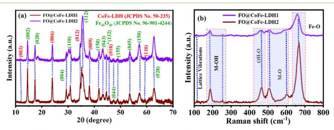
Fig. 4 Combine (a) XRD spectra and (b) Raman spectra of FO@CoFe-LDH1 and FO@CoFe-LDH2.
