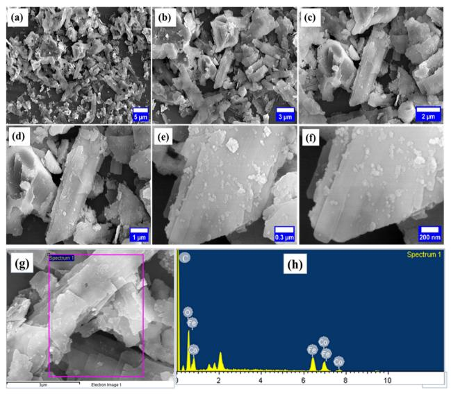
Fig. 2 FE-SEM images of FO@CoFe-LDH1 at 5 μm (a), 3 μm (b), 2 μm (c) 1 μm (d), 0.3 μm (e), 200 nm (f), (g) SEM image of FO@CoFe-LDH1 at 3 μm and (h) EDS spectra of FE-SEM image of Fig. 2(g).
