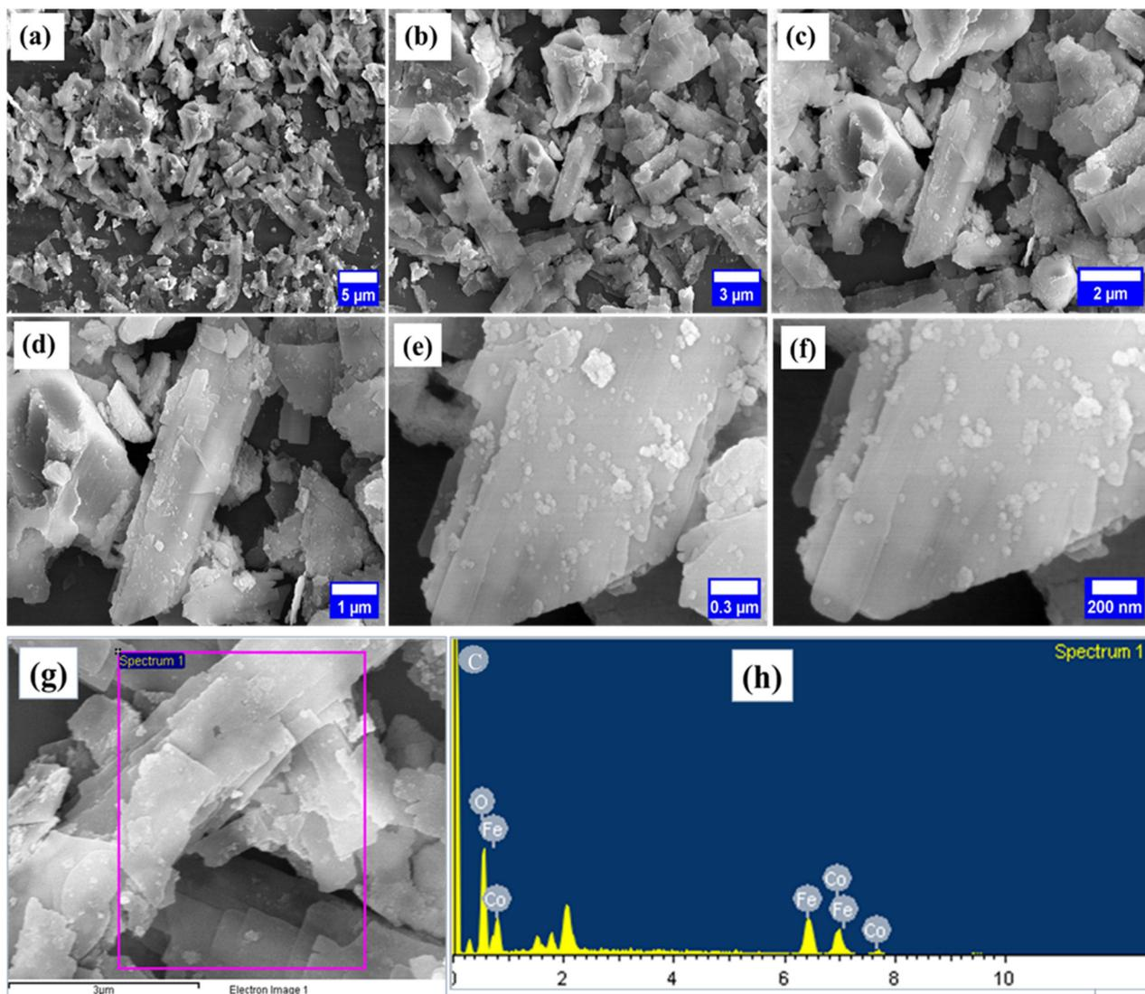
Fig. 2 FE-SEM images of FO@CoFe-LDH1 at 5  $\mu$ m (a), 3  $\mu$ m (b), 2  $\mu$ m (c) 1  $\mu$ m (d), 0.3  $\mu$ m (e), 200 nm (f), (g) SEM image of FO@CoFe-LDH1 at 3  $\mu$ m and (h) EDS spectra of FE-SEM image of Fig. 2(g).
