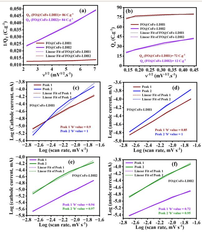
Fig. 8 (a and b) Trasatti methods for FO@CoFe-LDH1 and FO@CoFe-LDH2; (c and d) log (scan rates, mV s<sup>-1</sup>) vs. log (cathode current, mA) and log (scan rates, mV s<sup>-1</sup>) vs. log (anode current, mA) of FO@CoFe-LDH1, and (e and f) log (scan rates, mV s<sup>-1</sup>) vs. log (cathode current, mA) and log (scan rates, mV s<sup>-1</sup>) vs. log (anode current, mA) of FO@CoFe-LDH2.
