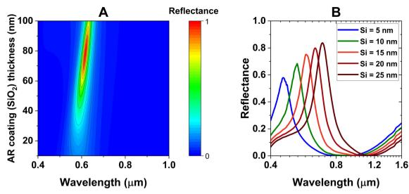
Fig. 5 (A) Contour plot showing reflectance variation as a function of AR coating (SiO<sub>2</sub>) thickness for the structure: Ag (100 nm)-SiO<sub>2</sub> (10 nm)-Si (15 nm)-SiO<sub>2</sub> (80 nm)-Ti (10 nm)-AR layer. (B) Reflectance spectra in the visible and NIR ranges for the same structure with varying Si thicknesses (5-25 nm) and fixed AR coating thickness (80 nm).
