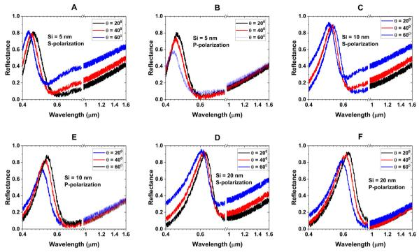
Fig. 7 Measured reflectance spectra of the Ag (100 nm)-SiO<sub>2</sub> (10 nm)-Si (5, 10, and 20 nm)-SiO<sub>2</sub> (80 nm)-Ti (10 nm) structure under oblique incidence. Panels (A, C and D) show S-polarized light, and (B, E and F) show P-polarized light for Si thicknesses of 5 nm, 10 nm, and 20 nm, respectively, at angles of 20°, 40°, and 60°.
