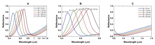
Fig. 3 Normal-incidence reflectance spectra for the MDSDM structure: Ag (100 nm)-SiO<sub>2</sub> (10 nm)-Si (5-25 nm)-SiO<sub>2</sub> (80 nm)-Ti (10 nm). (A) Shows the full spectral range across the visible and NIR regions. (B) Provides an expanded view of the visible range, while (C) shows an expanded view of the NIR region, corresponding to the regions in (A).
