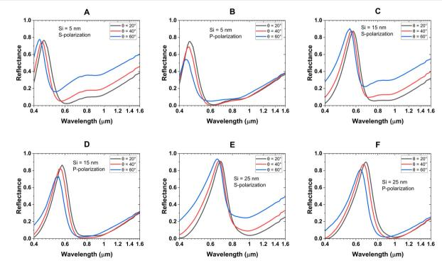
Fig. 4 Angle-dependent reflectance spectra of the Ag (100 nm)-SiO<sub>2</sub> (10 nm)-SiO<sub>2</sub> (80 nm)-Ti (10 nm) structure. Panels (A, C and E) show S-polarized results, and (B, D and F) show P-polarized results for Si thicknesses of 5 nm, 15 nm, and 25 nm, respectively, at incident angles of 20°, 40°, and 60°.
