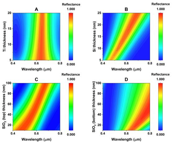
Fig. 2 Contour plots of calculated reflectance spectra in the visible range showing the effect of varying: (A) Ti layer thickness, (B) Si spacer thickness, (C) top SiO<sub>2</sub> thickness, and (D) bottom SiO<sub>2</sub> thickness.
