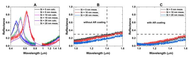
Fig. 8 (A and C) Calculated and measured reflectance spectra in the NIR region for the AR-coated structure: Ag (100 nm)-SiO<sub>2</sub> (10 nm)-SiO<sub>3</sub> (5, 10, and 20 nm)-SiO<sub>2</sub> (80 nm)-Ti (10 nm)-SiO<sub>3</sub> (80 nm). (B) Measured NIR reflectance spectra for the uncoated structure: Ag (100 nm)-SiO<sub>3</sub> (10 nm)-SiO<sub>4</sub> (10 nm)-SiO<sub>5</sub> (10 nm)-SiO<sub>6</sub> (10 nm)-SiO<sub>7</sub> (10 nm).
