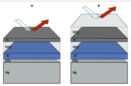
Fig. 1 Schematic diagrams of the proposed asymmetric Fabry-Perot nanocavity designs: (A) Ag-SiO<sub>2</sub>-Si-SiO<sub>2</sub>-Ti, representing the MDSDM configuration, and (B) Ag-SiO<sub>2</sub>-Si-SiO<sub>2</sub>-Ti-SiO<sub>2</sub>, representing the MDSDMD configuration.
