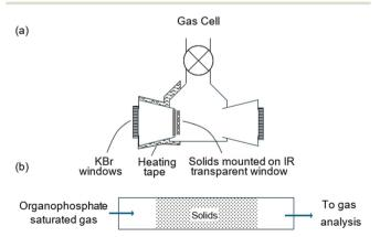
Fig. 4 Schematic diagram of (a) variable temperature infrared cell<sup>13,19,21</sup> (b) flow reactor setup containing powders<sup>8,40,49</sup> for studying vapor phase organophosphonates.
