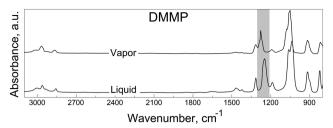
Fig. 5 Reference transmission FTIR spectra of vapor and liquid phases of  $\mathsf{DMMP}.^{64}$
