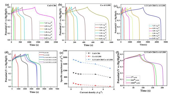
Fig. 7 GCD curves of (a) CuO-CB6, (b) Co-Al LDH, and (c) 1:2 CuO-CB6/Co-Al LDH in 1 M KOH at current densities of 7.27, 4.54, 1.81, 1.36, 0.90, and 0.45 A g<sup>-1</sup>. (d) GCD curves of CuO-CB6, Co-Al LDH, CuO-CB6/Co-Al LDH (1:2, 1:1, and 2:1) at 0.45 A g<sup>-1</sup>. (e) SC vs. current density plots of CuO-CB6, Co-Al LDH, and 1:2 CuO-CB6/Co-Al LDH attained from GCD. (f) GCD curve of 1:2 CuO-CB6/Co-Al LDH at the 2nd, 5000th, and 10 000th cycle at 7.27 A g<sup>-1</sup> current density.
