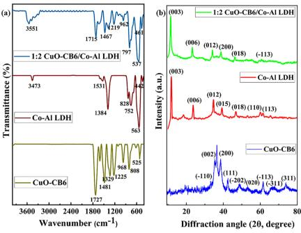
Fig. 2 (a) FT-IR and (b) XRD spectra of CuO-CB6, Co-Al LDH, and 1:2 CuO-CB6/Co-Al LDH.
