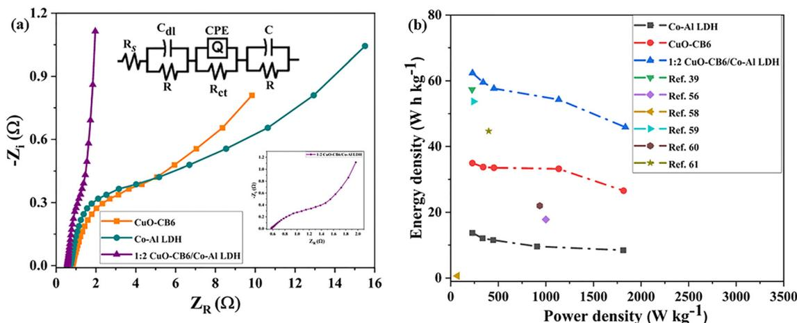
**Fig. 8** (a) Nyquist plots of CuO-CB6, Co-Al LDH, and 1:2 CuO-CB6/Co-Al LDH with the equivalent circuit diagram. (b) Ragone plot of CuO-CB6, Co-Al LDH, and 1:2 CuO-CB6/Co-Al LDH compared with other similar materials in the literature.
