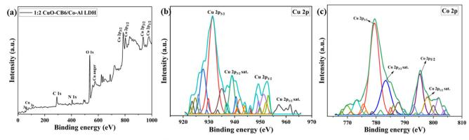
Fig. 5 (a) Wide scan XPS spectra of 1:2 CuO-CB6/Co-Al LDH & deconvolution peaks of (b) Cu 2p and (c) Co 2p.
