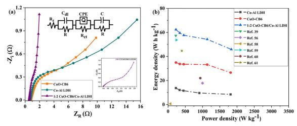
Fig. 8 (a) Nyquist plots of CuO-CB6, Co-Al LDH, and 1:2 CuO-CB6/Co-Al LDH with the equivalent circuit diagram. (b) Ragone plot of CuO-CB6, Co-Al LDH, and 1:2 CuO-CB6/Co-Al LDH compared with other similar materials in the literature.
