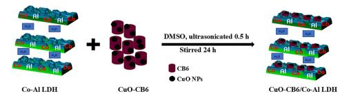
Fig. 1 Synthetic pathway of the CuO-CB6/Co-Al LDH nanocomposite.
