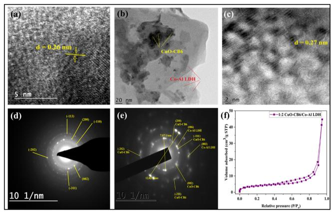
Fig. 4 HR-TEM micrograph of (a) CuO-CB6, (b and c) 1:2 CuO-CB6/Co-Al LDH, and SAED patterns of (d) CuO-CB6 & (e) 1:2 CuO-CB6/Co-Al LDH. (f) N<sub>2</sub> adsorption/desorption isotherm of 1:2 CuO-CB6/Co-Al LDH.
