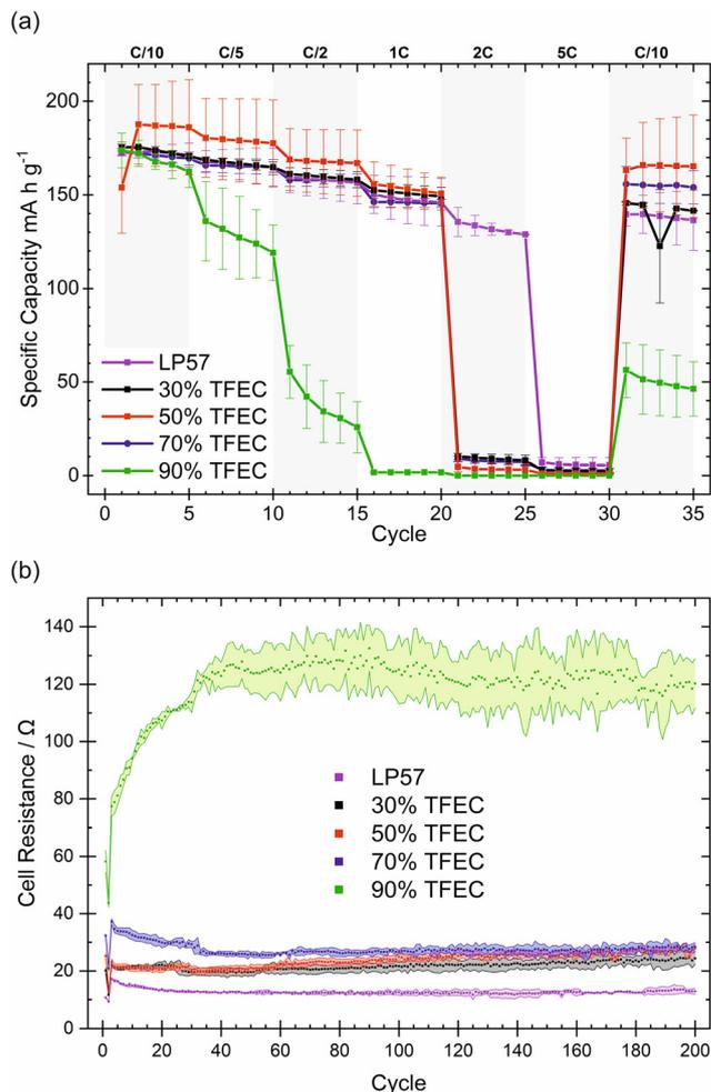
**Fig. 2** (a) Rate capability (discharge capacity) of TFEC containing electrolytes compared to LP57. (b) Internal resistance of the cell derived from the ICI measurement recorded at C/2. The resistance values are the averaged charge step for each cycle. The shaded area represents the standard deviation for two cells.
