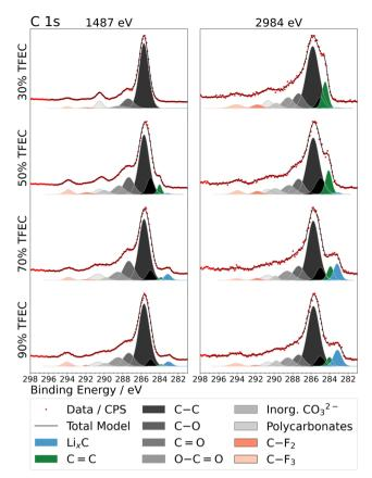
Fig. 3  $\,$  C 1s X-ray photoelectron spectra, measured at two excitation energies, for graphite electrodes cycled to 4 cycles in electrolytes with up to 90% TFEC.
