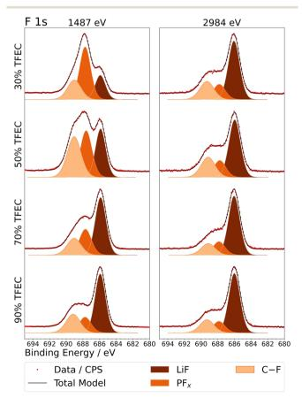
Fig. 4 F 1s X-ray photoelectron spectra, measured at two excitation energies, for graphite electrodes cycled to 4 cycles in electrolytes with up to 90% TFEC.
