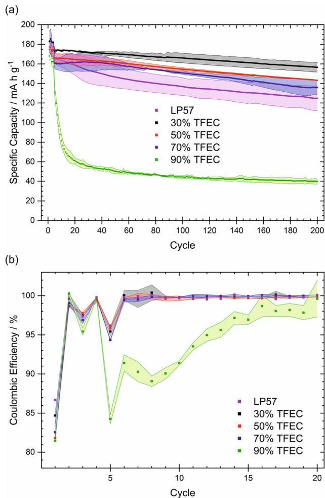
**Fig. 1** Electrochemical performance of NMC622/graphite cells with electrolytes containing up to 90% TFEC. (a) Galvanostatic cycling (discharge) over 200 cycles. (b) Coulombic efficiency over 20 cycles. The shaded areas represent the standard deviation of duplicate cells. The erratic coulombic efficiencies during the first five cycles are an artefact of increases in the C-rate.
