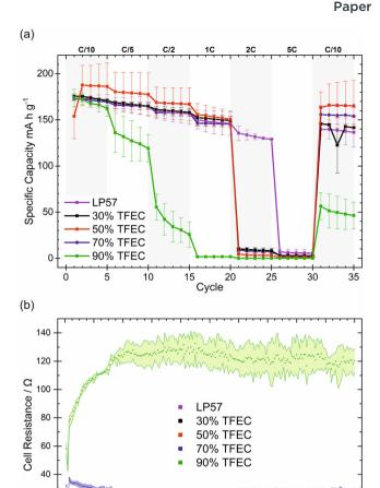
Fig. 2 (a) Rate capability (discharge capacity) of TFEC containing electrolytes compared to LP57. (b) Internal resistance of the cell derived from the ICI measurement recorded at C/2. The resistance values are the averaged charge step for each cycle. The shaded area represents the standard deviation for two cells.
