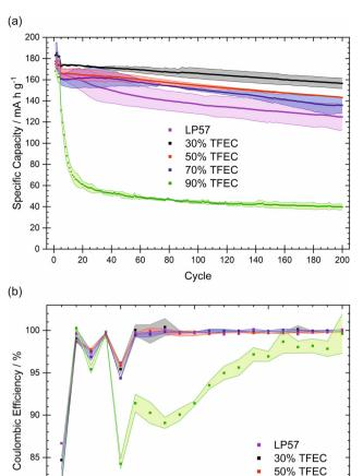
Fig. 1 Electrochemical performance of NMC622|graphite cells with electrolytes containing up to 90% TFEC. (a) Galvanostatic cycling (discharge) over 200 cycles. (b) Coulombic efficiency over 20 cycles. The shaded areas represent the standard deviation of duplicate cells. The erratic coulombic efficiencies during the first five cycles are an artefact of increases in the C-rate.
