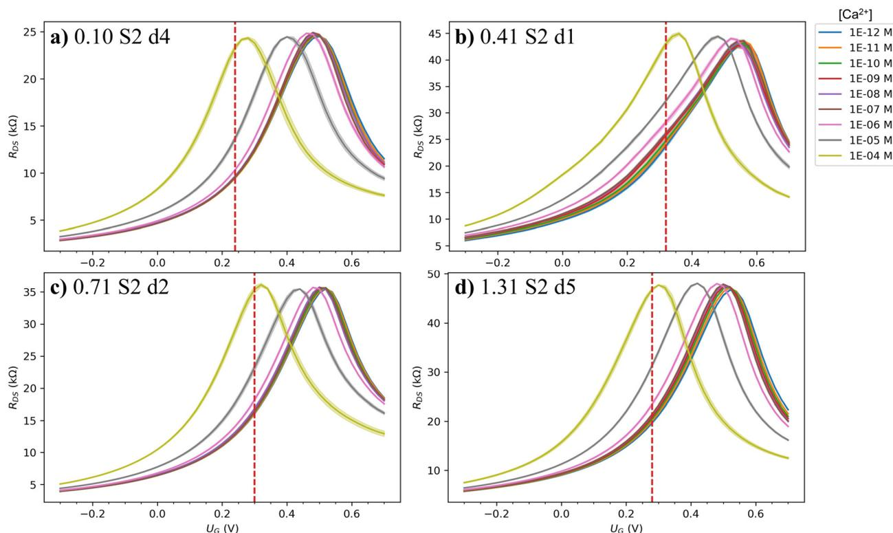
**Fig. 4** The  $R_{DS}$  transfer curves for Run 1 of four different oxidation level devices on the same substrate with their  $I_D/I_G$  ratios shown. The red vertical dashed lines indicate the  $U_G$  at which the maximum  $\Delta R_{DS}$  (i.e. the maximum response) was found for each measurement. See ESI† for full corresponding data of all the devices.
