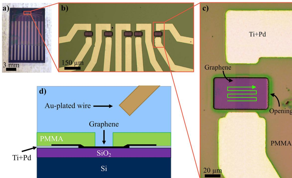
**Fig. 1** Optical images of a) a sample, b) all devices of one sample, and c) an individual device, where the 2P0 irradiation pattern is illustrated with a bright green arrow and d) a cross-sectional schematic of the geometry of the solution-gated measurements, where the Ti + Pd leads were the source and drain and the Au-plated Ag wire worked as the gate electrode.
