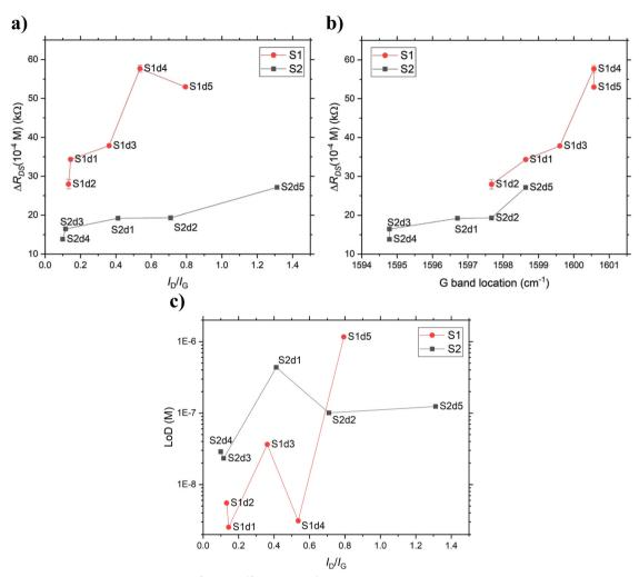
Fig. 6 The difference in resistance between  $[Ca^{2+}] = 10^{-12}$  M and  $10^{-4}$  M depicting the sensitivity as a function of a) the  $I_D/I_G$  ratio and b) the Raman shift of the G band and c) the estimated LoD as a function of the  $I_D/I_G$  ratio for each device of both substrates in Run 1. See ESI† for corresponding plots for the other measurement runs.
