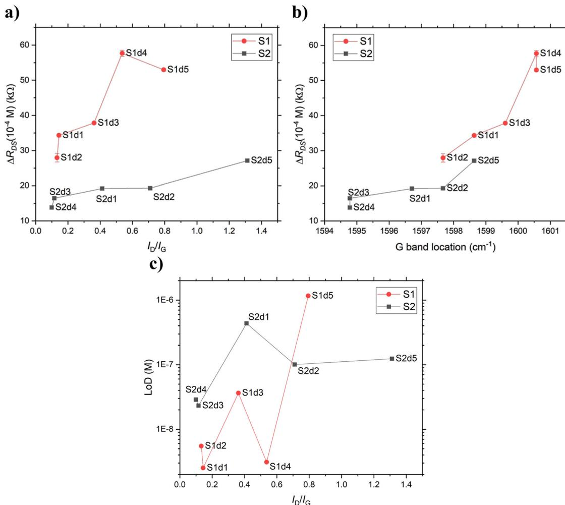
Fig. 6 The difference in resistance between  $[\text{Ca}^{2+}] = 10^{-12} \text{ M}$  and  $10^{-4} \text{ M}$  depicting the sensitivity as a function of a) the  $I_D/I_G$  ratio and b) the Raman shift of the G band and c) the estimated LoD as a function of the  $I_D/I_G$  ratio for each device of both substrates in Run 1. See ESI† for corresponding plots for the other measurement runs.
