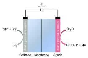
Fig. 1 Schematic illustration of a water electrolyzer. Copyright 2020, the Royal Society of Chemistry.
