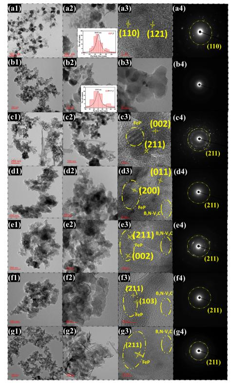
Fig. 4 The morphological analysis showing TEM, HRTEM and SAED pattern images of (a1–a4) pure  $V_2C$  (inset: particle size histogram), (b1–b4) B, N-V<sub>2</sub>C (inset: particle size histogram), and (c1–c4) FeP and (d1–d4) 5%, (e1–e4) 10%, (f1–f4) 15%, and (g1–g4) 20% wt. ratios of FeP@B,N-V<sub>2</sub>C nanostructures.
