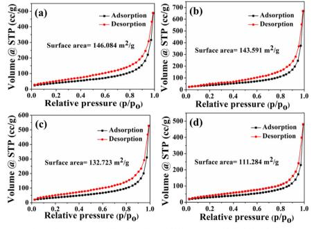
Fig. 5 (a-d) Nitrogen adsorption-desorption isotherms of 5%, 10%, 15%, and 20% wt. ratios of FeP@B,N-V<sub>2</sub>C nanostructures, respectively.
