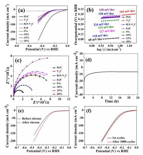
Fig. 8 (a) Polarisation curves for the HER. (b) Tafel plots and (c) EIS curves of FeP@B,N-V<sub>2</sub>C heterostructures and pure FeP and B,N-V<sub>2</sub>C NPs. (d) Chronoamperometry (i-t) studies and comparison of polarisation curves (e) before and after chronoamperometry and (f) 1000 CV cycles of the 10% FeP@B,N-V2C heterostructure
