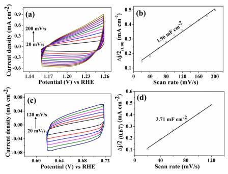
Fig. 7 Cyclic voltammograms and linear fit plots for (a and c) the OER and (b and d) HER at different scan rates from 20 mV s<sup>-1</sup> to 200 mV s<sup>-1</sup> of the 10% FeP@B,N- $V_2$ C nanostructure, respectively.
