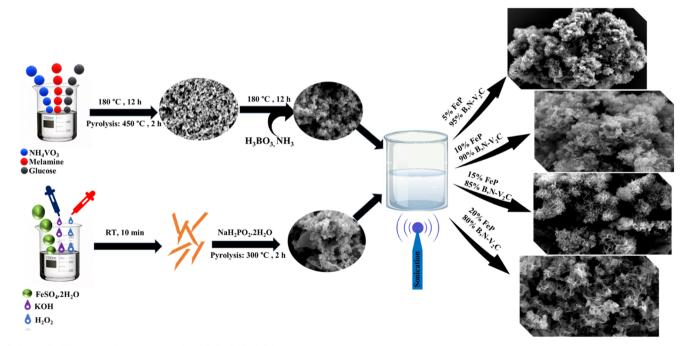
Scheme 1 Illustration for the synthesis of FeP@B,N-V2C heterostructures.
