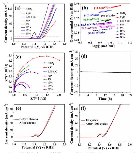
Fig. 6 (a) Polarisation curves for the OER. (b) Tafel plots and (c) EIS curves of FeP@B,N-V2C heterostructures and pure FeP and B,N-V<sub>2</sub>C NPs. (d) Chronoamperometry (i-t) studies and comparison of polarisation curves (e) before and after chronoamperometry and (f) 1000 CV cycles of the 10% FeP@B,N-V2C heterostructure.
