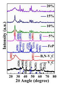
Fig. 1 The PXRD patterns of pure V<sub>2</sub>C, B,N-V<sub>2</sub>C, pure FeP, and the composite FeP@B,N-V2C nanomaterials (5%, 10%, 15%, 20% ratios).
