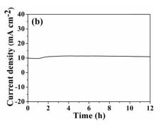
Fig. 9 (a) Polarization curves. (b) Chronoamperometry plot at an applied voltage of 1.57  $V@j_{10}$  mA cm<sup>-2</sup> for the 10% FeP@B,N-V<sub>2</sub>C||10% FeP@ V<sub>2</sub>C as the anode and cathode for overall water splitting in 1 M KOH.
