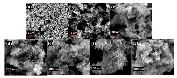
Fig. 3 The morphological analysis showing high magnification FESEM images of (a) pure V<sub>2</sub>C, (b) B,N-V<sub>2</sub>C, (c) FeP and (d) 5%, (e) 10%, (f) 15%, and (g) 20% wt. ratios of B,N-V<sub>2</sub>C@FeP nanostructures.
