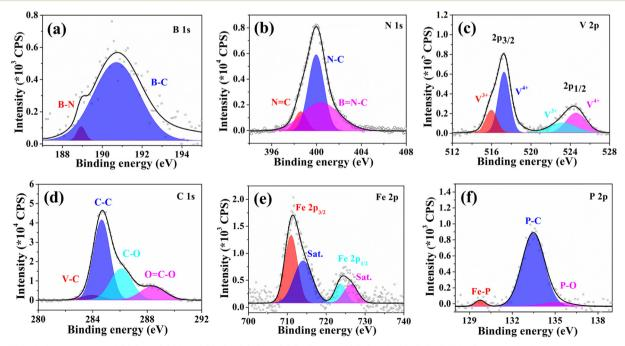
Fig. 2 XPS binding energies of (a) B 1s, (b) N 1s, (c) V 2p, (d) C 1s, (e) Fe 2p, and (f) P 2p of 10% FeP@B,N-V<sub>2</sub>C, respectively.
