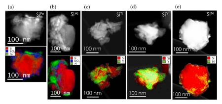
Fig. 1 STEM images and the corresponding electron energy loss spectroscopy (EELS) maps (red corresponds to Si, blue to SiO<sub>2</sub>, and green to the metal) of a) Si<sup>Fe</sup> b) Si<sup>Al</sup>, c) Si<sup>Ti</sup> d) Si<sup>Y</sup>, and e) Si<sup>Ni</sup> (see Fig. S1a† for Si<sup>Ag</sup>).
