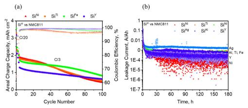
Fig. 11 a) Full cell cycling behavior of selected Si<sup>M</sup> with NMC811 at a C/3 rate and b) leakage current of Si<sup>M</sup> vs. NMC811 during charge at 4.1 V.
