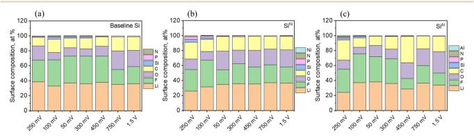
Fig. 10 Surface composition (at%) during lithiation at 250 mV, 100 mV, and 50 mV and \*delithiation at 300 mV, 450 mV, 750 mV, and 1.5 V of the a) baseline Si, b) Si<sup>Ni</sup>, and c) Si<sup>Al</sup> in half-cells. \*The electrodes were lithiated to 50 mV before delithiation.
