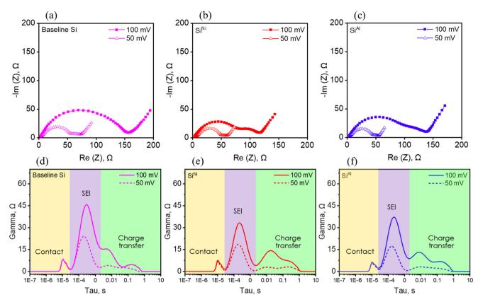
Fig. 9 Electrochemical impedance spectroscopy (EIS) Nyquist profiles at different lithiation potentials of a) baseline Si, b)  $Si^{Ni}$ , c)  $Si^{Ni}$ , c)  $Si^{Ni}$ , and the corresponding distribution of relaxation times (DRT) plots of d) baseline Si, e)  $Si^{Ni}$ , and f)  $Si^{Ni}$  within the 1 kHz to  $\sim$ 1 Hz frequency regime.
