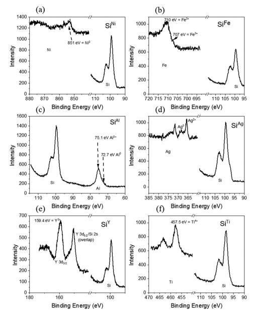
Fig. 2 High-resolution XPS spectra of the metal-decorated Si powders, specifically a) Si<sup>Ni</sup>, b) Si<sup>Fe</sup>, c) Si<sup>AI</sup>, d) Si<sup>Ag</sup>, e) Si<sup>Vi</sup>, and f) Si<sup>TI</sup>. The metal content of the samples is 10% as described in the experimental section.
