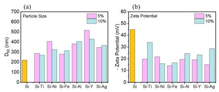
Fig. 4 a) Particle size ( $D_{50}$ ) of the metal-decorated Si powders measured by dynamic light scattering and their b) zeta potential in NMP solvent measured by phase angle light scattering analysis.
