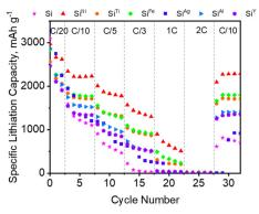
Fig. 7 Half-cell performance of the milled Si<sup>M</sup> (M: Ni, Ti, Fe, Ag, Al, Y) in Gen 2 + 3 wt% FEC electrolyte at room temperature at different C-rates (1C is based on 3579 mAh g<sup>-1</sup> for Li<sub>15</sub>Si<sub>4</sub>).
