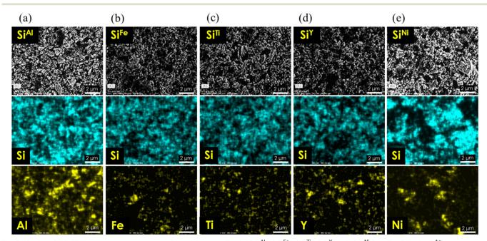
Surface SEM-EDX images of the decorated Si particles, specifically a) Si<sup>AI</sup>, b) Si<sup>Fe</sup>, c) Si<sup>Ti</sup>, d) Si<sup>Y</sup>, and e) Si<sup>Ni</sup> (see Fig. S1b† for Si<sup>Ag</sup>).
