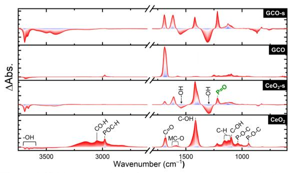
Fig. 2 DRIFTS spectra under DFP dosing over four aerogels variants. Spectra are recorded at 1 min intervals and progress from blue to red.
