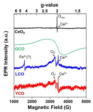
Fig. 6 Normalized EPR spectra of CeO<sub>2</sub>, GCO, YCO, and LCO aerogels. LCO and YCO show significant ROS (O2:-) signals, likely obscured in GCO due to the broad, wavy EPR lines.
