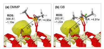
Fig. 5 Structures of (a) DMMP and (b) GB on the (111) CeO<sub>2</sub> surface, co-adsorbed with  $O_{\text{vac}}$ -stabilized ROS (purple). In each subfigure, the Bader basin computed for the ROS is shown in yellow and annotated with corresponding volume and partial charge. The Bader volume of the ROS, and likewise the ROS-P distance, is significantly larger for DMMP than GB.
