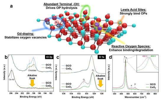
Fig. 1 (a) Schematic of GCO showing features for OP binding/degradation. (b) XPS Cl 2p region and (c) XPS O1s region for CeO2 and GCO aerogels before and after the alkaline soak. (d) Raman spectroscopy with inset showing the shift and broadening of the F<sub>2a</sub> peak.
