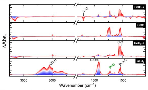
Fig. 3 DRIFTS spectra under a N<sub>2</sub> + O<sub>2</sub> purge after DFP exposure. Spectra are recorded at 1 min intervals and progress from blue to red.
