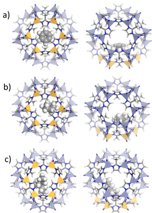
**Fig. 4** Location of a) benzene, b) cyclohexane and c) *n*-hexane molecules within ZIF-8\_ $CH_3$  structure using energy minimization approach through GCMC calculation. Orange polyhedra represent the zinc cations delimiting the 6MR windows in ZIF-8\_ $CH_3$  cavities.
