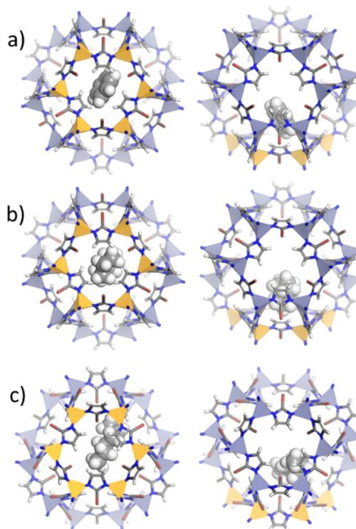
**Fig. 5** Location of a) benzene, b) cyclohexane and c) *n*-hexane molecules within ZIF-8\_Br structure using energy minimization approach through GCMC calculation. Orange polyhedra represent the zinc cations delimiting the 6MR windows in ZIF-8\_Br cavities.
