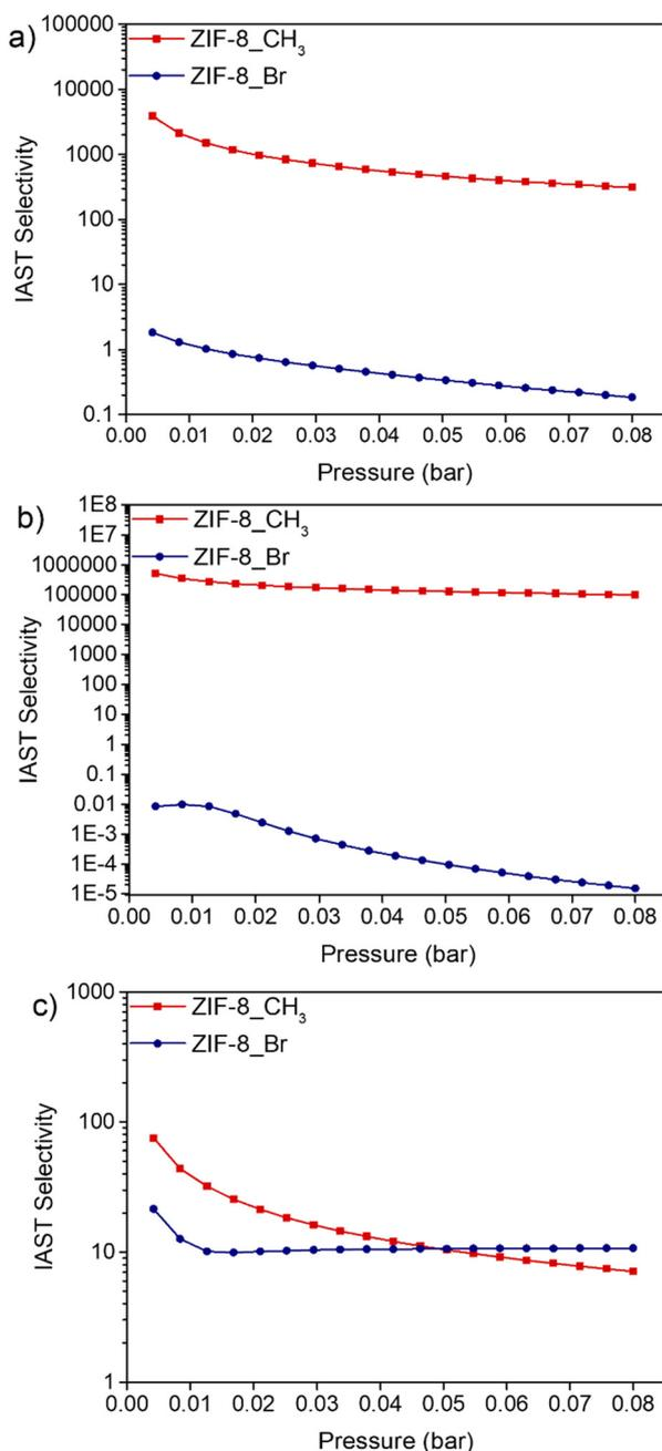
Fig. 6 IAST selectivities of VOC pairs at 293 K for ZIF-8\_CH<sub>3</sub> and ZIF-8\_Br including equimolar mixtures of a) *n*-hexane/cyclohexane, b) *n*-hexane/benzene and c) benzene/cyclohexane.
