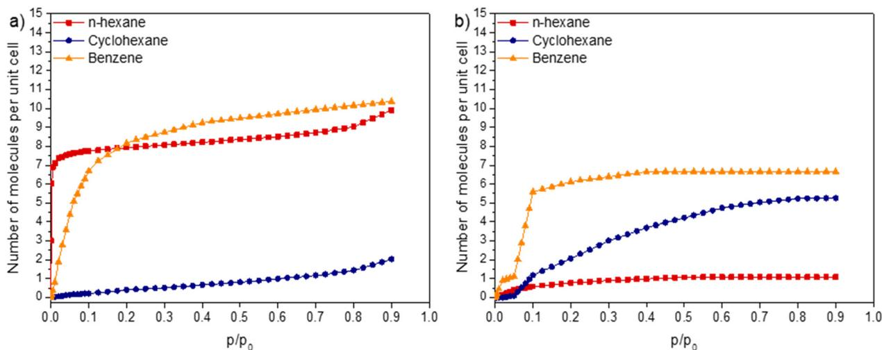
Fig. 1 Hydrocarbon adsorption isotherms at 293 K for a) ZIF-8-CH<sub>3</sub> and b) ZIF-8-Br.
