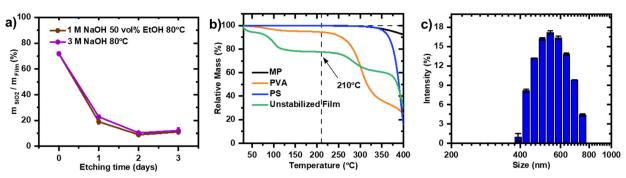
Fig. 1 a) Tracking the etching of SiO<sub>2</sub> from the carbon support in alkaline solutions by measuring the residual SiO<sub>2</sub> after oxidative burn off of the carbon with TGA in compressed air (CA) atmosphere. b) TGA of MP, PVA, PS and unstabilized film in nitrogen (N2) atmosphere. c) Particle size distribution of synthesized PS spheres.
