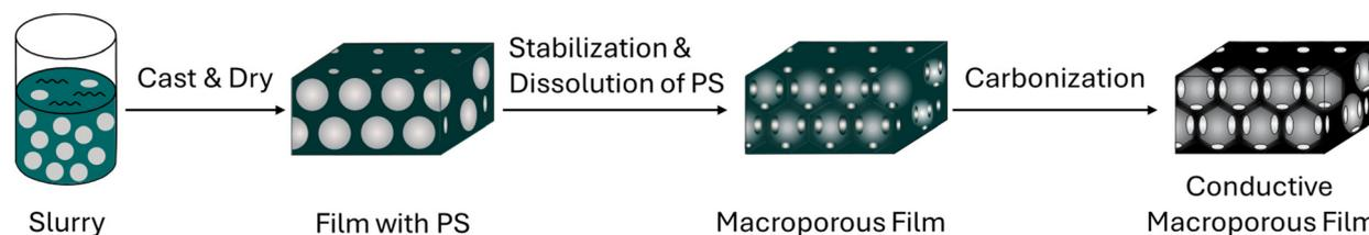
Scheme 1 Preparation steps for the conductive macroporous film.
