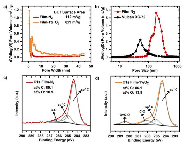
Fig. 3 a) Pore size distribution in for micro- and mesopore range obtained by nitrogen adsorption before electrochemical characterization. b) Pore size distribution for cathodes based on Film- $N_2$  and Vulcan XC-72/Sustainion obtained by MIP before electrochemical characterization. XPS spectra of the C1s for the film carbonized in c)  $N_2$  and in d)  $1\% O_2/99\% N_2$  before electrochemical characterization.
