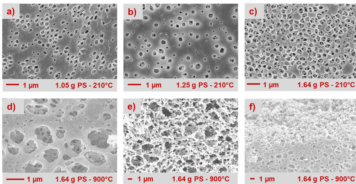
**Fig. 2** Upper row: Films with different proportions of PS a) 1.05 g, b) 1.25 g and c) 1.64 g after the oxidative stabilization step at 210 °C and subsequent dissolution of the PS template. Bottom row: Film with 1.64 g PS carbonized at 900 °C with d) top view, e) cross section view and f) edge view.
