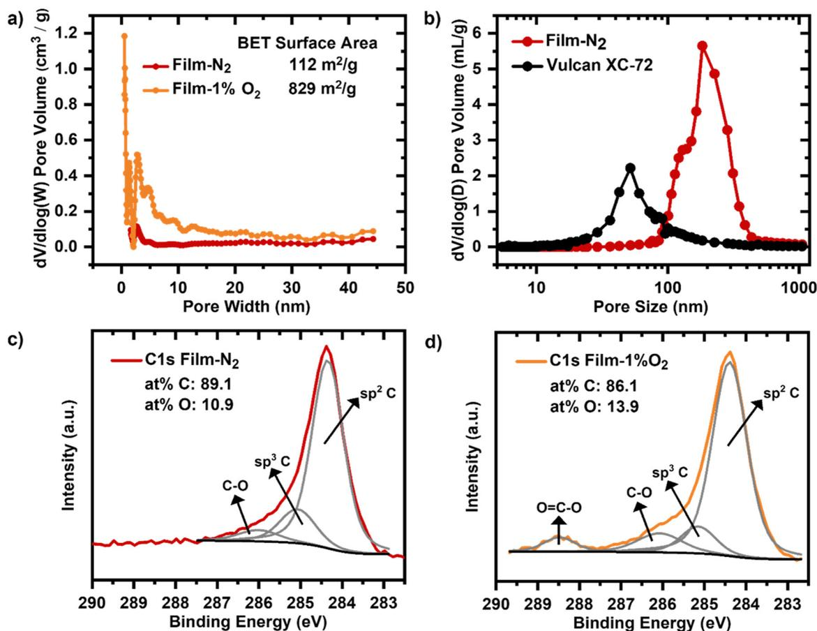
Fig. 3 a) Pore size distribution in for micro- and mesopore range obtained by nitrogen adsorption before electrochemical characterization. b) Pore size distribution for cathodes based on Film-N<sub>2</sub> and Vulcan XC-72/Sustainion obtained by MIP before electrochemical characterization. XPS spectra of the C1s for the film carbonized in c) N<sub>2</sub> and in d) 1% O<sub>2</sub>/99% N<sub>2</sub> before electrochemical characterization.
