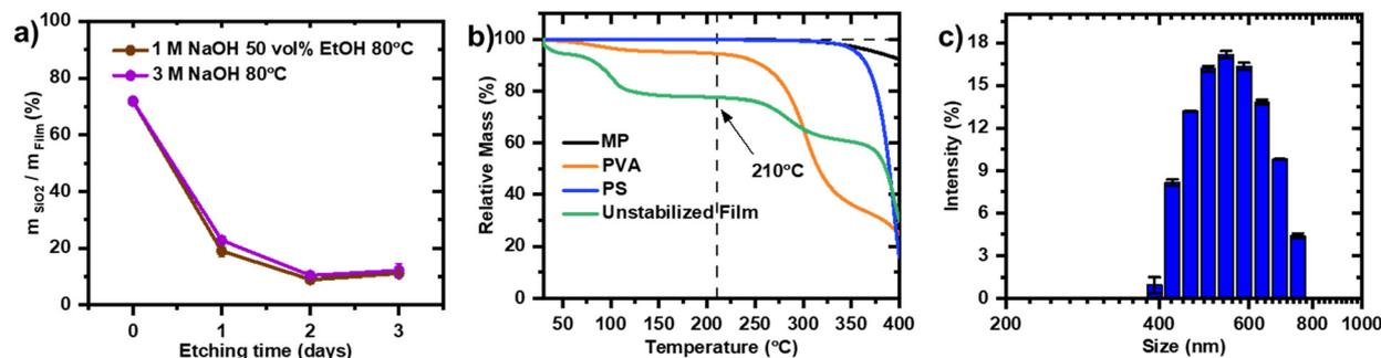
**Fig. 1** a) Tracking the etching of SiO<sub>2</sub> from the carbon support in alkaline solutions by measuring the residual SiO<sub>2</sub> after oxidative burn off of the carbon with TGA in compressed air (CA) atmosphere. b) TGA of MP, PVA, PS and unstabilized film in nitrogen (N<sub>2</sub>) atmosphere. c) Particle size distribution of synthesized PS spheres.
