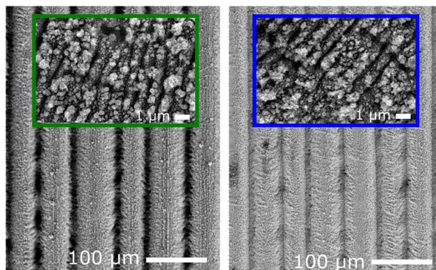
**Fig. 5** Scanning electron micrographs of the laser-processed surfaces extracted from two opposite corners of the beam screen. The inserts visualize the nanofeatures on top of the ridges of the formed surface topography.
