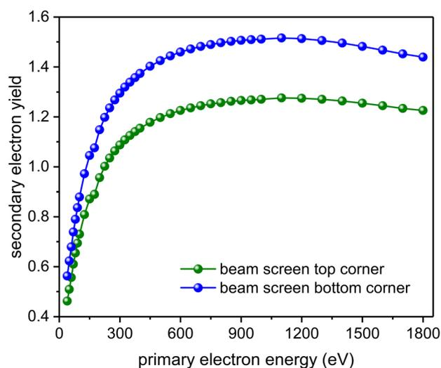
**Fig. 6** Room temperature secondary electron yield of two samples extracted from opposite corners of the selectively-treated beam screen (average of three measured spots). The corresponding SEM images are plotted in Fig. 5.
