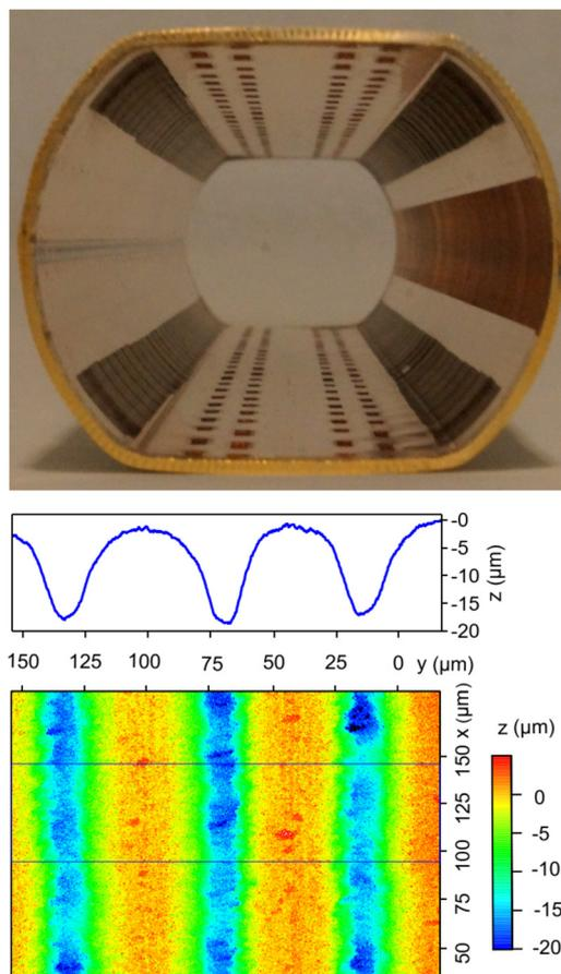
**Fig. 4** Top: Cross-sectional photograph of the 40 cm long beam screen after finalization of the selective laser treatment. Four regions of 20° azimuthal width each at the corners were laser-processed and appear dark, while untreated regions remain bright. The band in the center right is the sawtooth profile for reduction of synchrotron light reflection (see text for more information). Bottom: Line profile and 2D map of the laser-structured surface topography.
