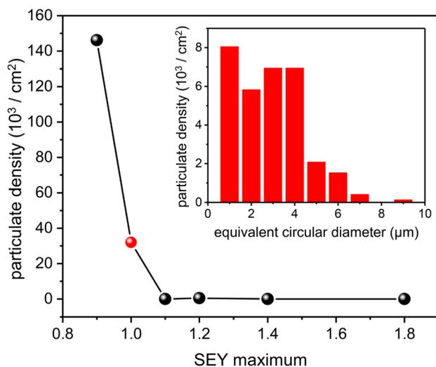
Fig. 7 Summary of centrifugation tests applying a force density of  $3 \text{ N mm}^{-3}$ . The graph shows the number of detached particles per unit area as a function of the maximum SEY of the laser treated surface. The size-distribution of the equivalent diameter of collected particles for the case of the surface with SEY maximum of 1.0 (red data point) is shown in the inset.
