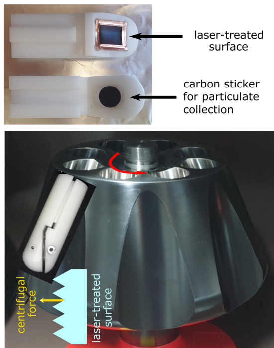
Fig. 2 Experimental setup for particulate detachment tests. Top row: Photograph of disassembled sample holder. Bottom row: Rotor with installed sample holder and schematic of centrifugal force acting on the laser-treated surface.
