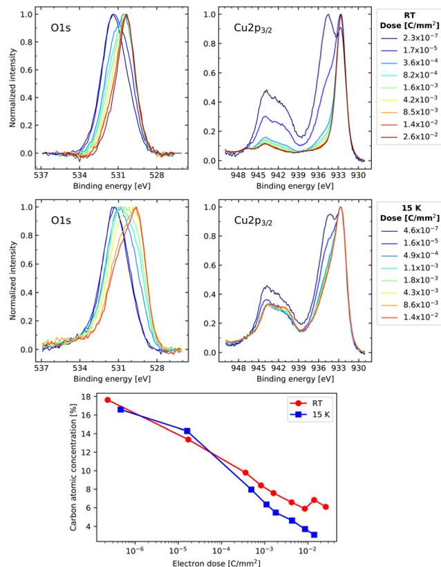
**Fig. 9** Chemical surface analysis by XPS during the room temperature and cryogenic electron-conditioning of laser-treated Cu surfaces with initial  $\delta_{\text{max}} = 1.4$ . Top and middle: Background-subtracted O 1s and Cu 2p<sub>3/2</sub> core level spectra after exposure to increasing electron doses at room temperature and 15 K, respectively. Bottom: Reduction of the surface carbon content during the electron-induced transformation processes.
