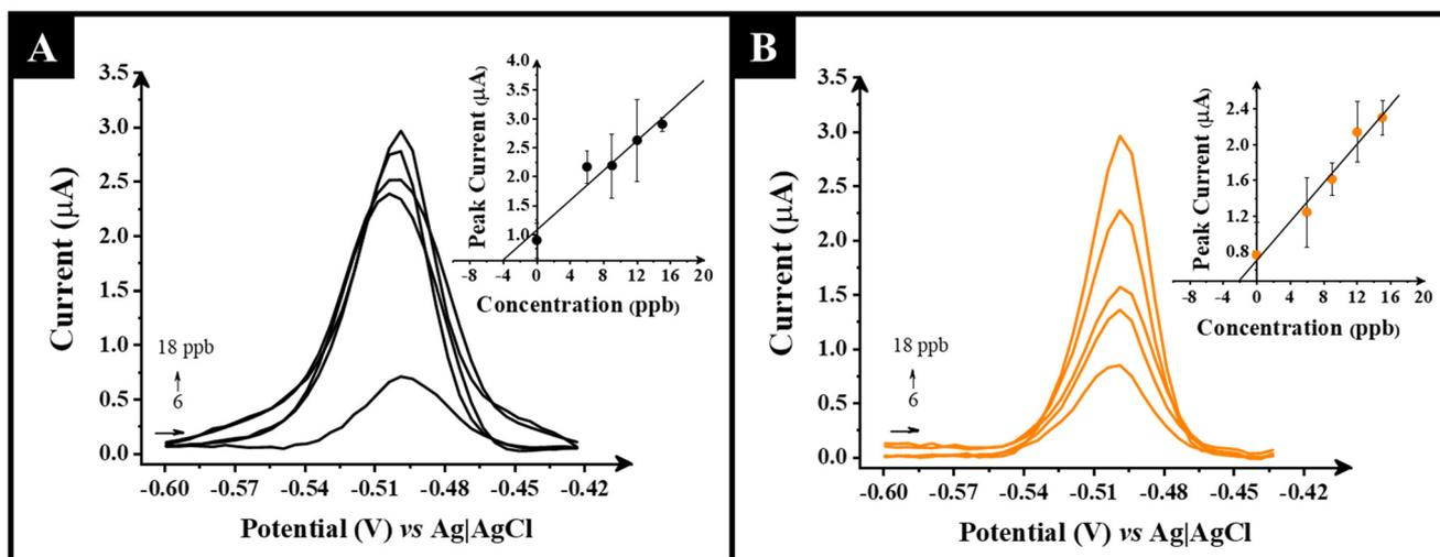
Fig. 5 SWASV for  $\text{Pb}^{2+}$  in diluted river water (50-fold) in HCl 0.1 M performed at (A) graphite and (B) AuNP-G electrodes in a concentration range of 6 to 18 ppb (6, 9, 12, 15, and 18 ppb). SWASV parameters:  $a = 60 \text{ mV}$ ,  $f = 40 \text{ Hz}$ ,  $\Delta E = 9 \text{ mV}$ ,  $E_{\text{deposition}} = -1.1 \text{ V}$ , and  $t_{\text{deposition}} = 120 \text{ s}$ . Insets: calibration curves obtained by the standard addition method.
