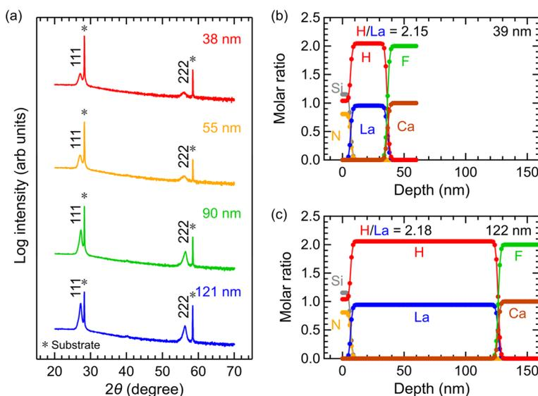
**Fig. 1** (a)  $2\theta$ - $\omega$  X-ray diffraction patterns of LaH<sub>2</sub> epitaxial thin films with different film thicknesses. Depth profiles of the chemical composition of the (b) 39- and (c) 122 nm-thick LaH<sub>2</sub> films with SiN<sub>x</sub> capping layers grown on CaF<sub>2</sub> substrates. The zero depth corresponds to the surface of the SiN<sub>x</sub> capping layer.
