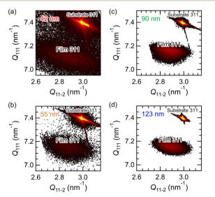
Fig. 2 (a)-(d) Reciprocal space mappings near the 311 diffraction for  $LaH_2$  epitaxial thin films with thicknesses of (a) 42, (b) 55, (c) 90, and (d) 123 nm.
