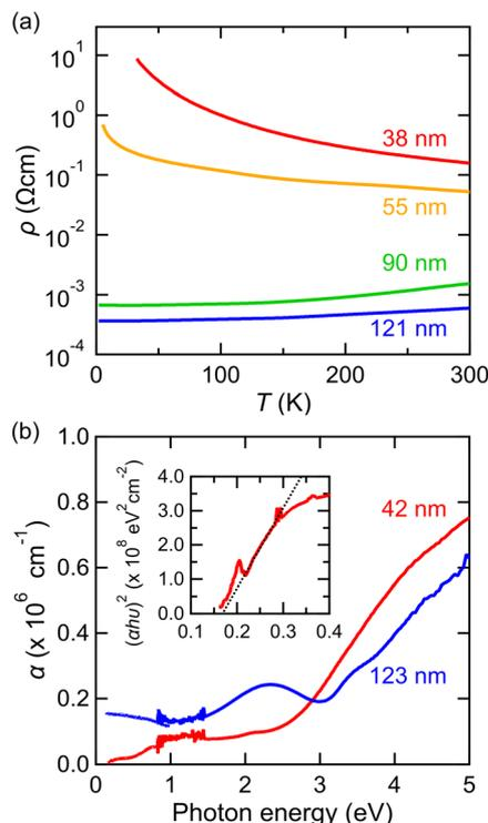
**Fig. 4** (a) Temperature dependence of electrical resistivity and (b) optical absorption spectra for LaH<sub>2</sub> epitaxial thin films with different thickness. The inset of (b) shows the Tauc plot of the absorption edge, where the dotted line denotes the fitting line to evaluate the band gap.
