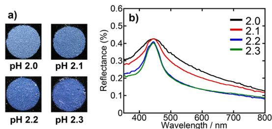
Fig. 4 a) Photographs and b) UV-vis reflectance spectra of PBs prepared from SiO<sub>2</sub> dispersions with pH values of 2.0, 2.1, 2.2, and 2.3.
