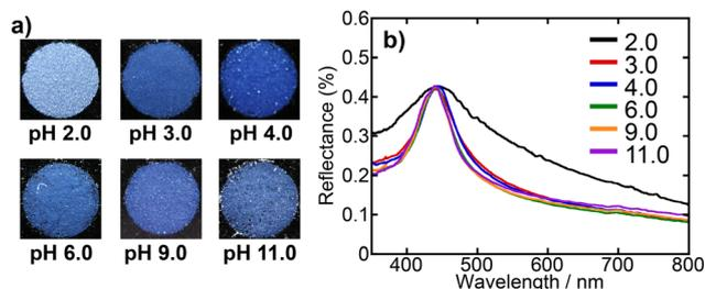
Fig. 3 a) Photographs and b) UV-vis reflectance spectra of PBs prepared from SiO<sub>2</sub> dispersions with pH values of 2.0, 3.0, 4.0, 6.0, 9.0, and 11.0.
