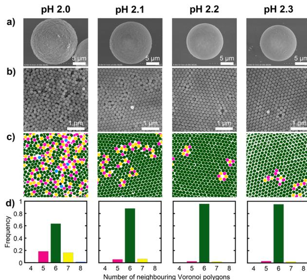
Fig. 5 SEM images of a) the entire spheres and b) surfaces of the PBs prepared from SiO<sub>2</sub> dispersions with pH values of 2.0, 2.1, 2.2, and 2.3. c) Voronoi diagrams obtained from SEM images and d) distributions of the number of neighbouring Voronoi polygons. Black: 4-fold polygons, pink: 5-fold polygons, green: 6-fold polygons, yellow: 7-fold polygons, blue: 8-fold polygons.
