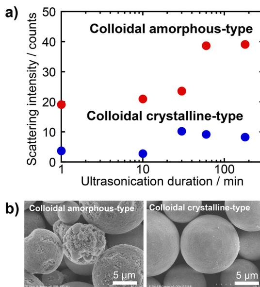
**Fig. 10** a) Changes in the light-scattering intensity of the PB dispersion as a function of the ultrasonication duration and b) SEM images of PBs with colloidal amorphous-type and colloidal crystalline-type arrangements after ultrasonic irradiation for 180 min.
