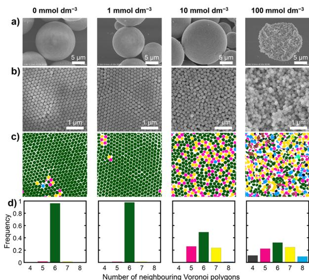
**Fig. 7** SEM images of a) the entire spheres and b) surfaces of the PBs prepared from  $\text{SiO}_2$  dispersions with  $\text{NH}_4\text{Cl}$  concentrations of 0, 1, 10, and  $100 \text{ mmol dm}^{-3}$ . c) Voronoi diagrams obtained from SEM images and d) distributions of the number of neighbouring Voronoi polygons. Black: 4-fold polygons, pink: 5-fold polygons, green: 6-fold polygons, yellow: 7-fold polygons, blue: 8-fold polygons.
