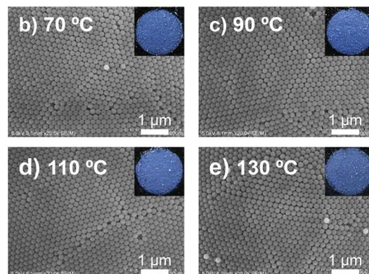
**Fig. 8** a) UV-vis reflectance spectra and b–e) surface SEM images of PBs prepared at drying temperatures of 70, 90, 110, and  $130 \text{ }^\circ\text{C}$  using  $\text{SiO}_2$  dispersions devoid of the ionic additive. Photographs of PBs are provided as insets in the SEM images.
