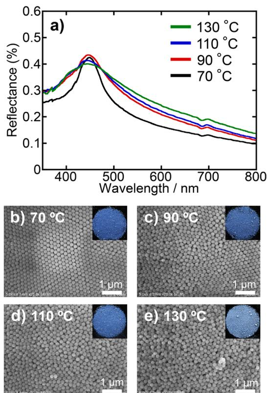
**Fig. 9** a) UV-vis reflectance spectra and b-e) surface SEM images of PBs prepared at drying temperatures of 70, 90, 110, and 130 °C using SiO<sub>2</sub> dispersions with NH<sub>4</sub>Cl (10 mmol dm<sup>-3</sup>). Photographs of PBs are provided as insets in the SEM images.
