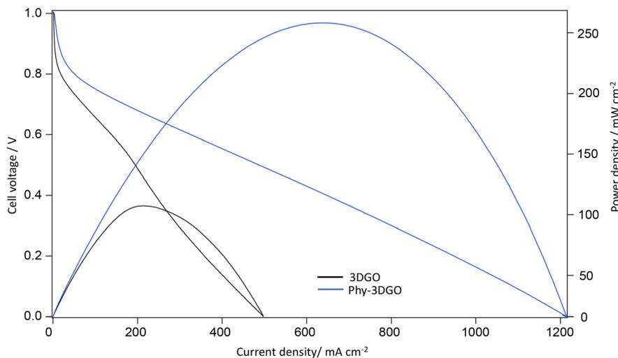
**Fig. 3** The single-cell performance evaluation using the 3DGO membrane and Phy-3DGO as the proton conducting electrolyte. *I*-*V* curves and power densities for the 3DGO and Phy-3DGO membrane fuel cells.
