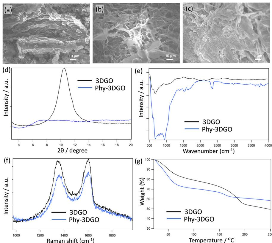
**Fig. 1** Morphological and chemical properties of 3DGO and Phy-3DGO. a) SEM image of 3DGO, b) SEM image of Phy-3DGO, c) cross-sectional SEM image of Phy-3DGO, d) PXRD of 3DGO and Phy-3DGO, e) FTIR of 3DGO and Phy-3DGO, f) Raman spectra of 3DGO and Phy-3DGO and g) TGA analysis of 3DGO and Phy-3DGO.
