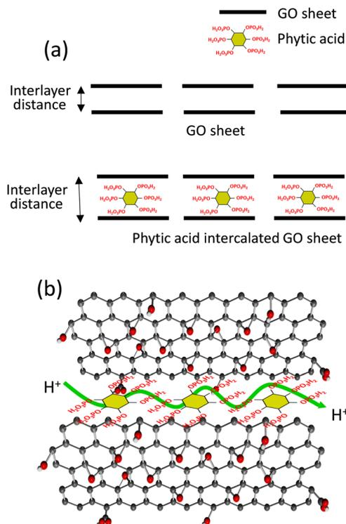
**Scheme 1** Phytic acid intercalated graphene oxide. a) Improvement in the interlayer distance due to the intercalation of phytic acid in GO and b) an expected better hydration pathway for improved proton conductivity in the phytic acid intercalated 3DGO.
