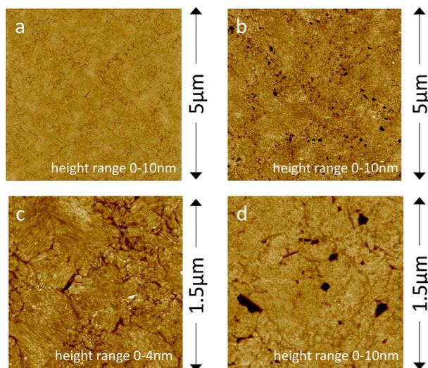
**Fig. 4** AFM images of template-stripped gold surfaces with a MH:HT (50:50) SAM (a and c) before and (b and d) after the formation of SSHM (0.5 mg mL<sup>-1</sup> per HV for 1 h at 20 °C, 10 mM CaCl<sub>2</sub>, 20 mM MOPS, 30 mM Na<sub>2</sub>SO<sub>4</sub>, pH 7.4).
