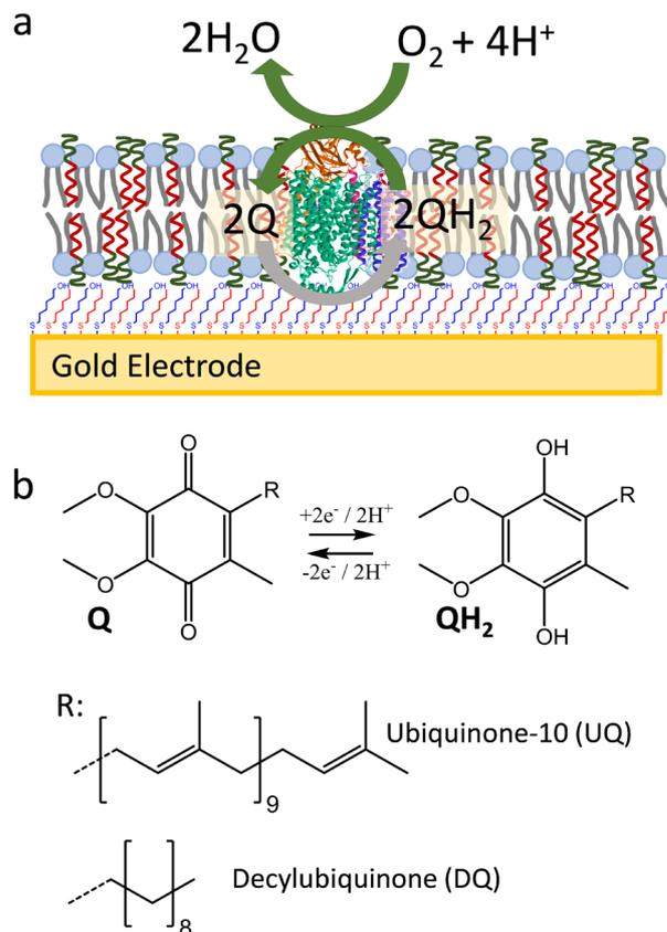
Fig. 1 (a) Schematic representation of cyt *bo*<sub>3</sub> in SSHM on gold electrode modified with a mixed SAM of MH:HT (1:1 molar ratio). In this system, ubiquinol is reduced at the electrode to ubiquinol, which is then reoxidized by cyt *bo*<sub>3</sub>, catalyzing oxygen reduction to water. (b) Structures of ubiquinone-10 (UQ) and decylubiquinone (DQ) in their fully oxidized (Q) and reduced forms (QH<sub>2</sub>).
