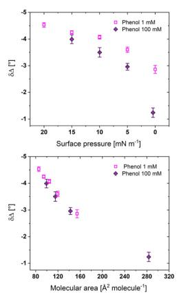
Fig. 4 Ellipsometric measurements of PL1 at the air-subphase interface as a function of phenol concentration in the supphase. Each value represents the average of measurements made on three independently formed films. For each independent film, the  $\delta\Delta$  is the average of 10 measurements of the same monolayer film at constant surface pressure.
