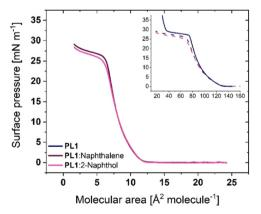
Fig. 5 Surface pressure-molecular area isotherms of PL1 and lipid mixtures with 1:10 molar ratio of PL1:naphthalene and PL1:2naphthol (solid lines, pressure onset area  $\sim$ 13  ${\rm \AA}^2$  molecule<sup>-1</sup>). Inset: the same isotherms are replotted as a function of pure phosphole-lipid molecular area (dashed lines).
