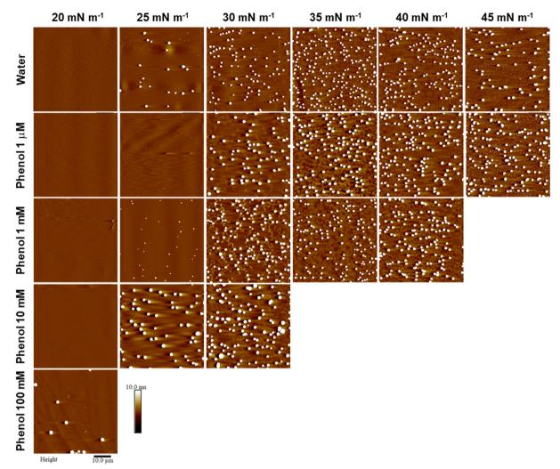
Fig. 3 Representative AFM images of PL1 deposited onto mica by LB at different surface pressures from water and phenol subphases (concentrations as indicated). All images are  $50 \times 50 \, \mu m^2$ , with height scale of 10 nm. The height scale was selected to enable visualization of the monolayer domains which are otherwise obscured by the large height of the aggregates (average aggregate heights are provided in Fig. S1†).
