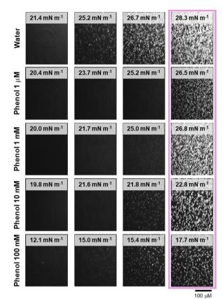
Fig. 2 Representative BAM images of PL1 on water and different subphase concentrations of phenol. The images corresponding to the surface pressures of the main phase transition plateau are aligned vertically and framed (pink).
