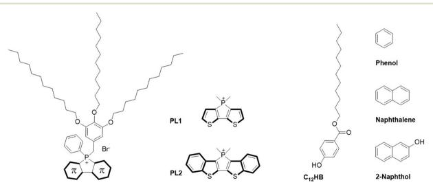
Scheme 1 Chemical structure of previously reported phosphole-lipid with dithienophosphole headgroup (PL1), phosphole-lipid with benzo-fused dithienophosphole headgroup (PL2),<sup>24</sup> dodecyl 4-hydroxybenzoate surfactant (C<sub>12</sub>HB), and the aromatic molecules phenol, naphthalene, and 2-naphthol
