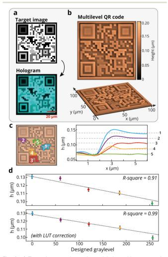
Fig. 4 a) Target image and experimental holographic pattern of a multilevel QR code. b) AFM micrographs of the azopolymer surface, measured immediately after the holographic exposure. c) Crosssectional profiles corresponding to the different topographical levels highlighted by the coloured domains in the AFM map. d) Measured average height distribution of coloured domains of the multilevel reliefs. The top and the bottom plots show the results before and after the LUT correction.
