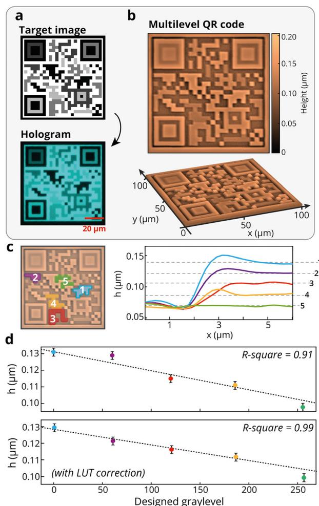
**Fig. 4** a) Target image and experimental holographic pattern of a multilevel QR code. b) AFM micrographs of the azopolymer surface, measured immediately after the holographic exposure. c) Cross-sectional profiles corresponding to the different topographical levels highlighted by the coloured domains in the AFM map. d) Measured average height distribution of coloured domains of the multilevel reliefs. The top and the bottom plots show the results before and after the LUT correction.
