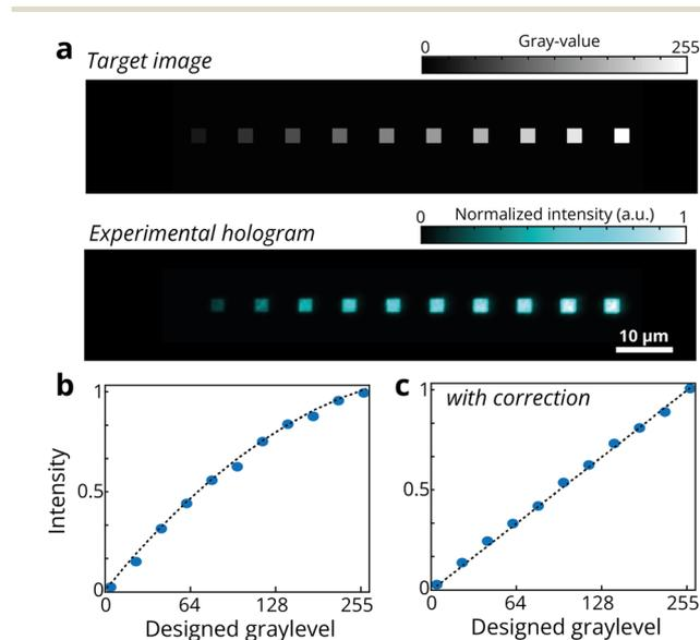
**Fig. 3** a) Target image and reconstructed holographic pattern to evaluate the optical system performance in terms of grayscale light modulation. b and c) Reconstructed intensity levels before and after the LUT correction, respectively.
