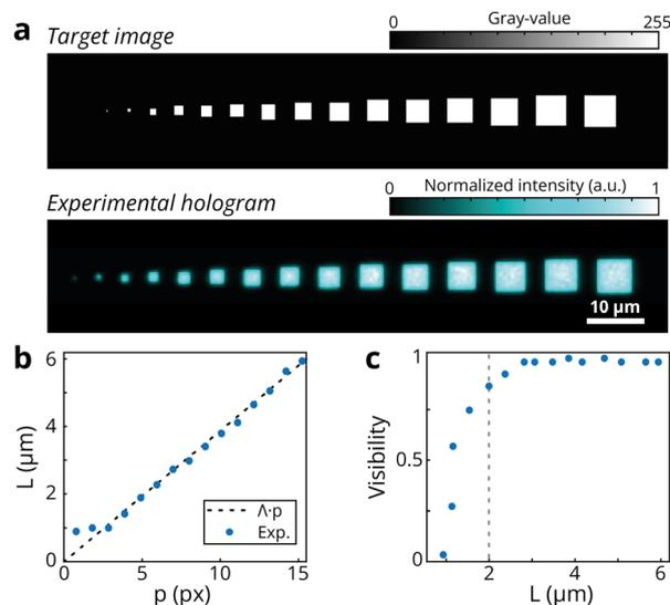
**Fig. 2** a) Target image and reconstructed holographic pattern to evaluate the resolution limit of the setup. b) Physical size of the squares  $L$  as a function of the designed size  $p$ . c) Visibility of the reconstructed squares as a function of their size  $L$ .
