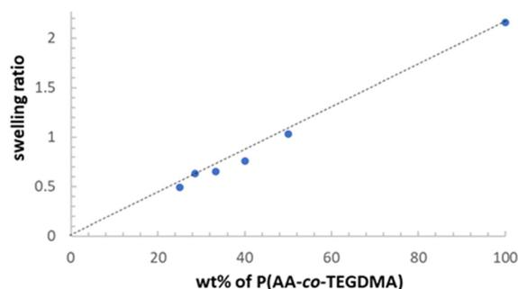
Fig. 9 Swelling ratios of PAA-based polymer/HNT composites and P(AA-co-TEGDMA).
