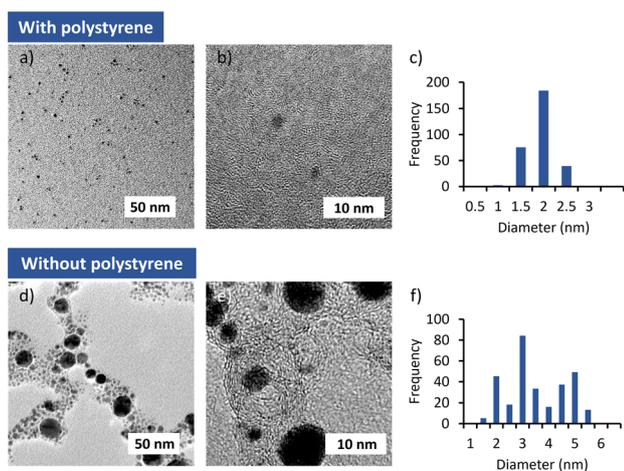
**Fig. 1** a), b), d) and e) TEM images and c) and f) size distribution of Au NCs prepared a)–c) under polystyrene and d)–f) in the absence of polystyrene. The applied average energy was 180 mW for each.
