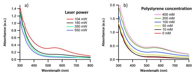
**Fig. 4** The UV-vis spectrum of carbon-encapsulated Au NCs obtained by using a) different laser powers in 50 mM polystyrene/toluene solution and b) different polystyrene concentrations with applying 104 mW average power. All the samples were prepared as 0.03 mM Au in THF.
