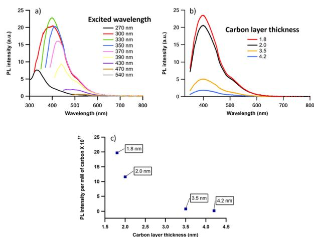
**Fig. 6** Emission properties of carbon-coated Au NCs obtained by PLAL using MCL in polystyrene/toluene mixture. a) Emission spectra of carbon-coated Au NCs excited at various wavelengths. b) Emission spectra of Au NCs with different carbon layer thicknesses. Excitation wavelength was 330 nm. c) Carbon layer thickness-PL intensity relationship. All the samples were prepared as 0.03 mM Au in THF.
