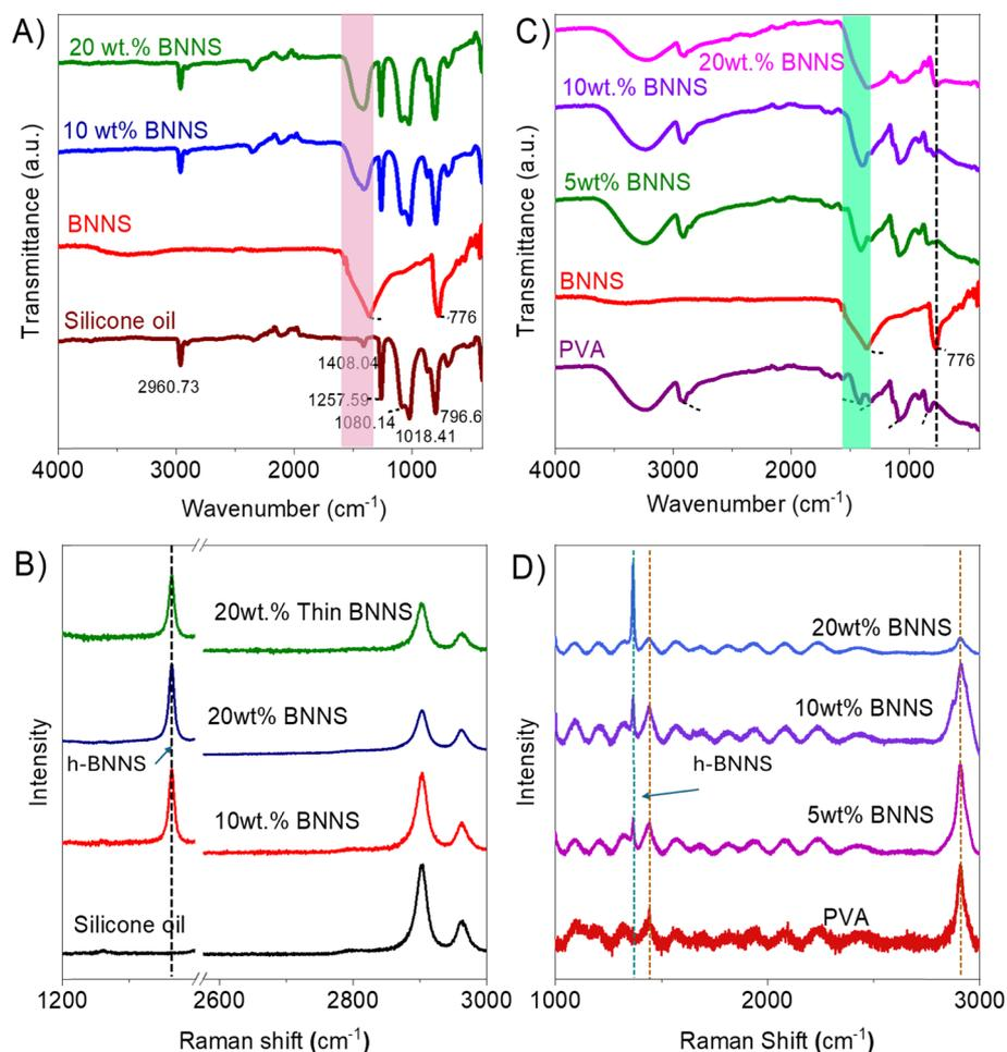
**Fig. 6** Investigation of interaction between the h-BN filler and matrix. A and B) Fourier-transform infrared spectra and Raman spectra of silicone oil-based thermal grease with different percentages of exfoliated h-BNNS and C and D) FTIR and Raman spectra of polyvinyl alcohol-based thermal film with different percentages of exfoliated h-BNNS.
