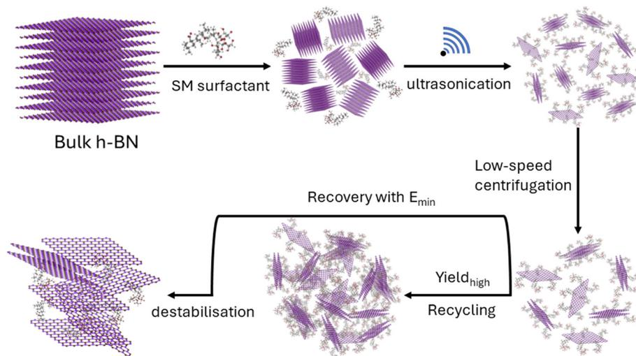
Fig. 1 Scheme for liquid-phase exfoliation and processing of bulk h-BN into few-layered h-BN nanosheets using a natural SM surfactant.
