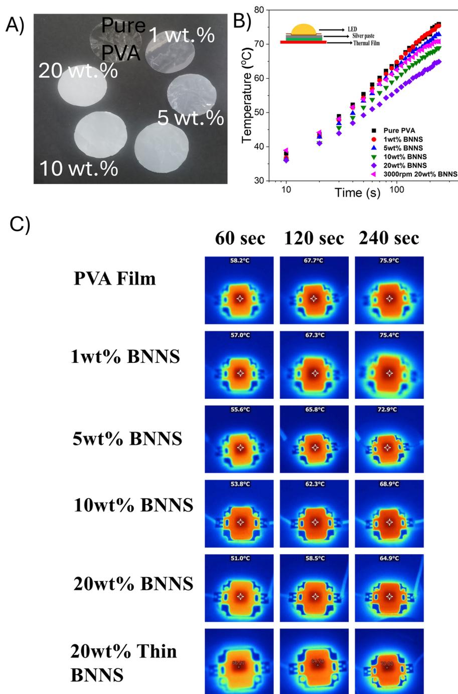
**Fig. 8** h-BNNS modified polymer film for thermal management. A) Photograph of bare PVA film and h-BNNS embedded thermal films with different weight percentages of the filler, B) progression of the surface temperature of the LED bulb (10 W) as a function of glowing time using different types of heat-spreading composite films (inset: architecture of the device for testing) and C) thermal infrared images of the LED bulb at specific intervals.
