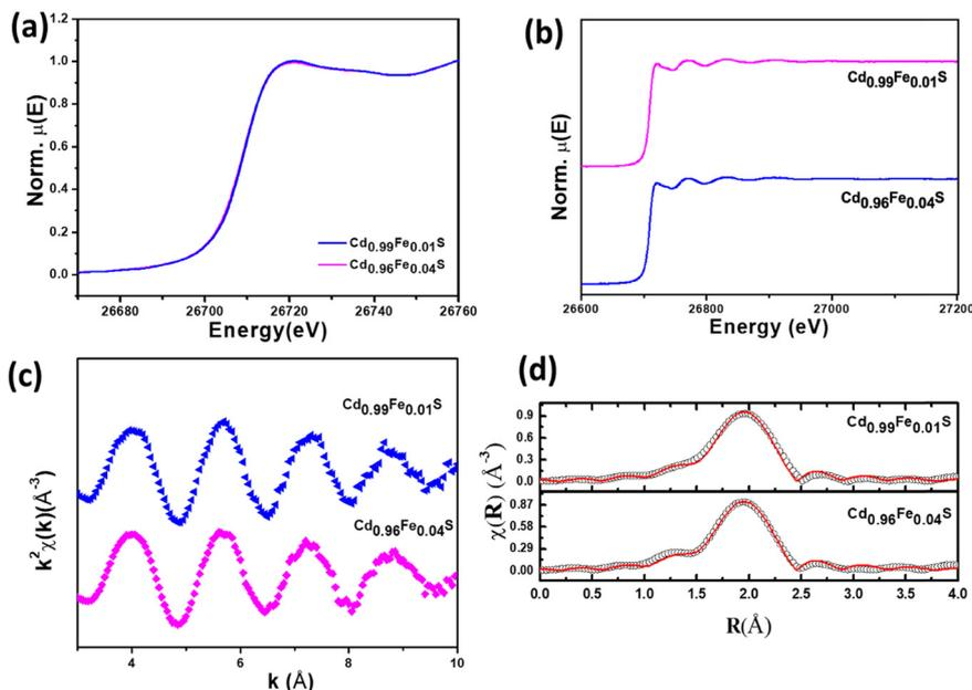
Fig. 4 (a) Normalized XANES spectra, (b) normalized absorption spectra, (c) normalised EXAFS ( $k^2\chi(k)$  vs.  $k$ ) spectra, and (d) Fourier-transformed EXAFS spectra of  $\text{Cd}_{0.99}\text{Fe}_{0.01}\text{S}$  and  $\text{Cd}_{0.96}\text{Fe}_{0.04}\text{S}$  quantum dots at the Cd K-edge. In (d), the black colored scatter points represent experimental spectra, and the red colored solid line represents the theoretical fit.
