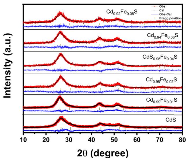
Fig. 1 Rietveld refinement profiles of X-ray diffraction (XRD) data of undoped and Fe-doped CdS quantum dots [ $\text{Cd}_{1-x}\text{Fe}_x\text{S}$ ,  $\text{Fe} = 0, 0.01, 0.02, 0.04, 0.06$ , and  $0.08$ ]. The experimental data are represented by 'Obs', and the theoretical fit by Rietveld refinement is represented by 'Cal'.
