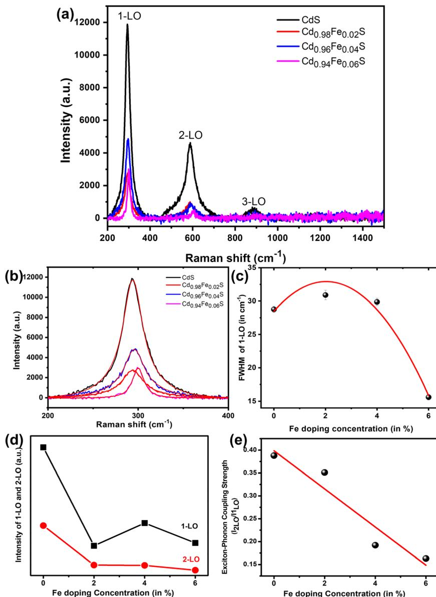
**Fig. 6** (a) Raman spectra of  $\text{Cd}_{1-x}\text{Fe}_x\text{S}$  quantum dots at room temperature, (b) Raman spectra of  $\text{Cd}_{1-x}\text{Fe}_x\text{S}$  quantum dots: 1-LO (fitted to get the exact peak position), (c) FWHM variation (1-LO) with Fe doping concentrations, (d) relative Raman intensity of 1-LO with increasing Fe doping concentrations, (e) variation in exciton-phonon coupling strength with Fe doping concentration.
