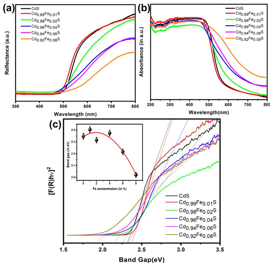
Fig. 7 (a) Reflectance spectra and (b) absorbance spectra of undoped and Fe-doped CdS quantum dots [Cd<sub>1-x</sub>Fe<sub>x</sub>S; Fe = 0%, 1%, 2%, 4%, 6%, and 8%]; (c) Tauc plots of undoped and Fe-doped CdS quantum dots (inset: band gap variation with Fe doping concentration).
