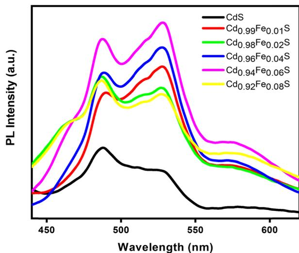
Fig. 8 Photoluminescence spectra of undoped and Fe-doped CdS [Cd<sub>1-x</sub>Fe<sub>x</sub>S] quantum dots.
