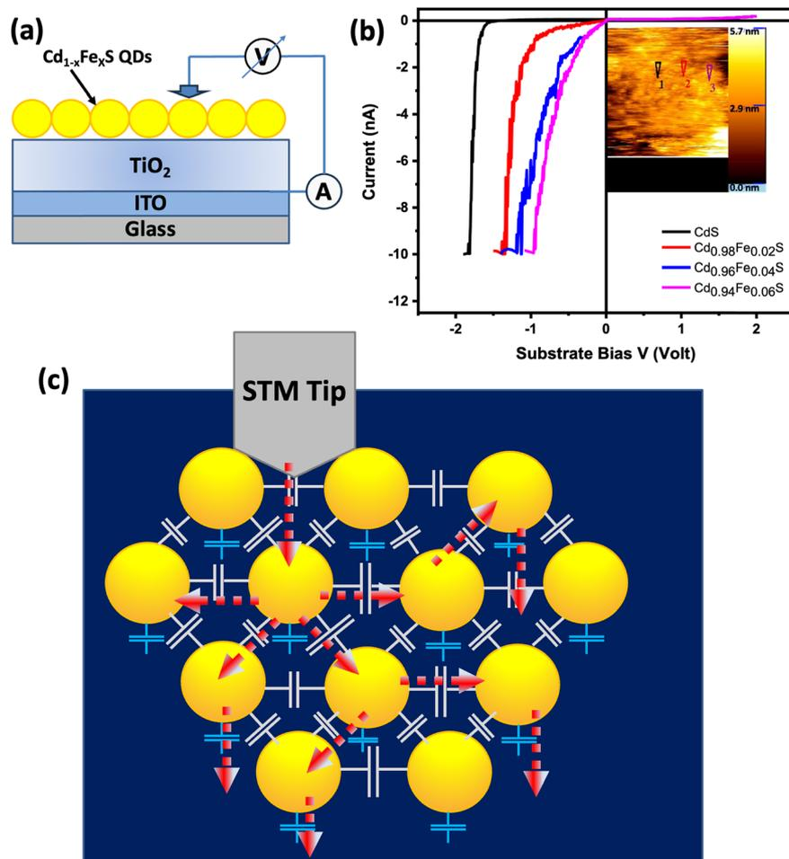
**Fig. 9** (a) Device structure of the ITO/TiO<sub>2</sub>/Cd<sub>1-x</sub>Fe<sub>x</sub>S QDs rectifying diode [Fe = 0%, 2%, 4%, and 6%] and (b) rectifying behaviors of undoped and Fe-doped CdS single quantum dots (inset shows the scanning tunneling micrograph of 2% Fe-doped CdS QDs). (c) Schematic of the model of collective transport phenomena in the device. The yellow spheres denote CdS QDs. The dashed red line with arrows illustrates the electron transport path.
