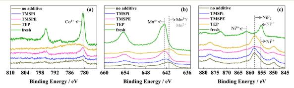
Fig. 5 The Co 2p (a), Mn 2p (b) and Ni 2p (c) XPS spectra of the cycled Li<sub>1.144</sub>Ni<sub>0.136</sub>Co<sub>0.136</sub>Mn<sub>0.544</sub>O<sub>2</sub> electrodes placed in the electrolytes with different additives.
