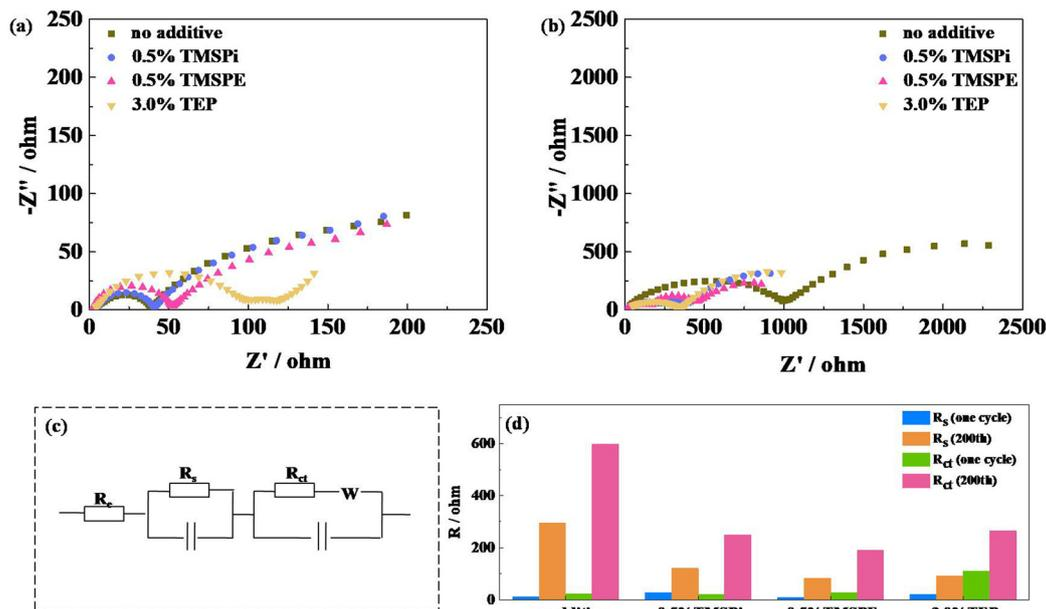
Fig. 3 Electrochemical impedance spectra of  $\text{Li}_{1.144}\text{Ni}_{0.136}\text{Co}_{0.136}\text{Mn}_{0.544}\text{O}_2/\text{Li}$  cells with different additive charged to 4.8 V after one cycle (a) and the 200 cycles (b); the equivalent circuit model used to analysis the EIS spectra (c) and the fitting result of  $R_s$  and  $R_{ct}$  of  $\text{Li}_{1.144}\text{Ni}_{0.136}\text{Co}_{0.136}\text{Mn}_{0.544}\text{O}_2/\text{Li}$  cells with electrolytes in the different additives (d).
