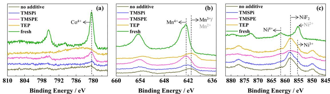
Fig. 5 The Co 2p (a), Mn 2p (b) and Ni 2p (c) XPS spectra of the cycled  $\text{Li}_{1.144}\text{Ni}_{0.136}\text{Co}_{0.136}\text{Mn}_{0.544}\text{O}_2$  electrodes placed in the electrolytes with different additives.
