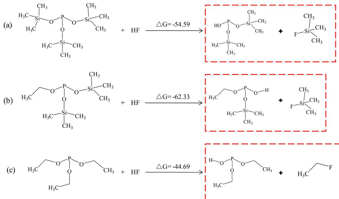
Fig. 6 Reaction energies ( $\Delta G$  in  $\text{kJ mol}^{-1}$ ) of (a) TMSPi, (b) TMSPE, and (c) TEP with a HF molecule.
