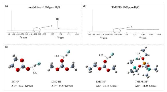
Fig. 8 (a and b) <sup>19</sup>F NMR spectra of the electrolytes with and without adding 0.5% TMSPE after storage under 25 °C for 24 h; (c) optimized structures and the relative combination energies (\( \Delta E \), kJ mol<sup>-1</sup>) between HF and solvents or an electrolyte additive: DMC/EC/EMC/TMSPE-HF.
