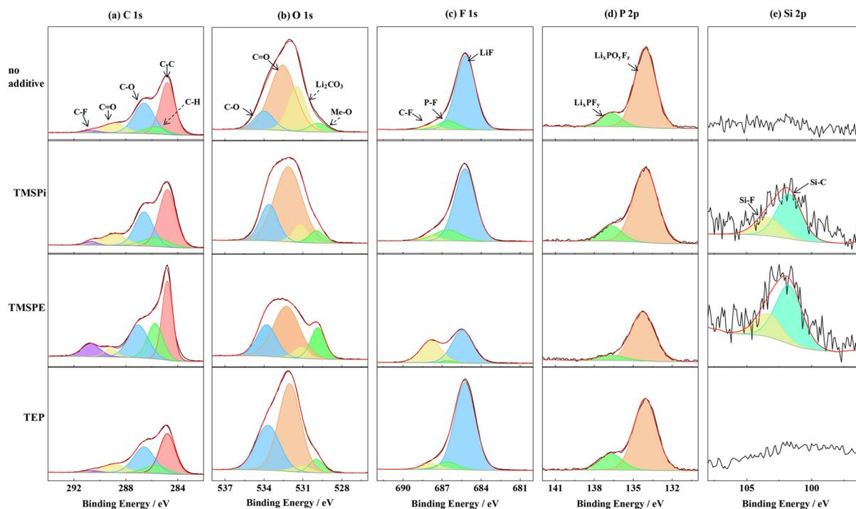
Fig. 4 C 1s (a), O 1s (b), F 1s (c), P 2p (d) and Si 2p (e) XPS spectra of the cycled  $\text{Li}_{1.144}\text{Ni}_{0.136}\text{Co}_{0.136}\text{Mn}_{0.544}\text{O}_2$  electrodes placed in the electrolytes with different additives.
