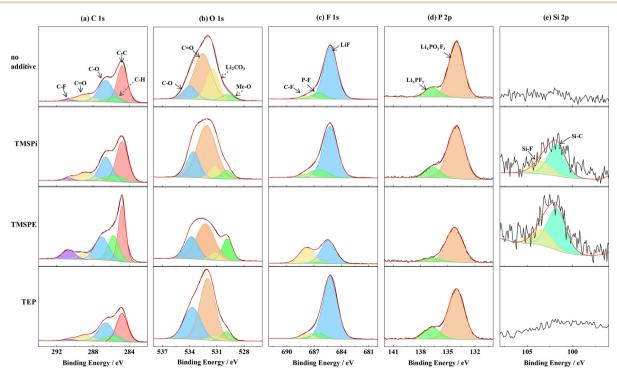
Fig. 4 C 1s (a), O 1s (b), F 1s (c), P 2p (d) and Si 2p (e) XPS spectra of the cycled  $Li_{1.144}Ni_{0.136}Co_{0.136}Mn_{0.544}O_2$  electrodes placed in the electrolytes with different additives
