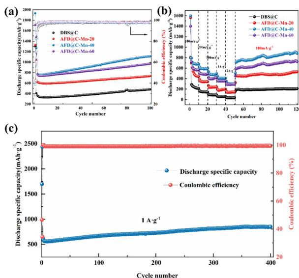
Fig. 7 (a) Long cycle performance and (b) gravimetric capacity *versus* cycle number at different current densities of DBS@C, AFD@C-Mn-20, AFD@C-Mn-40, and AFD@C-Mn-60. (c) Long-term cycling performance of AFD@C-Mn-40 at  $1 \text{ A g}^{-1}$ .
