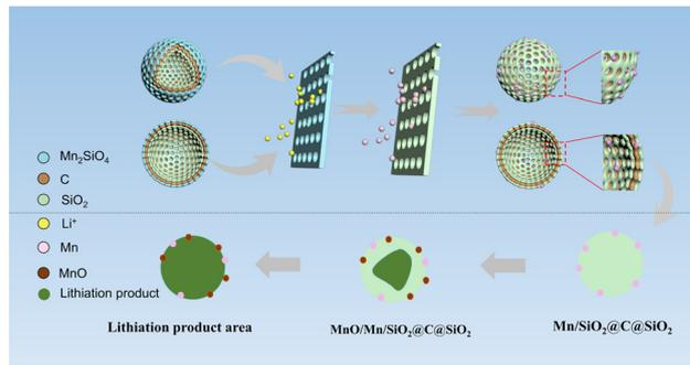
Fig. 9 Schematic diagram of the rapid activation mechanism of the Mn<sub>2</sub>SiO<sub>4</sub>@C@SiO<sub>2</sub> multilayer-structure composite.
