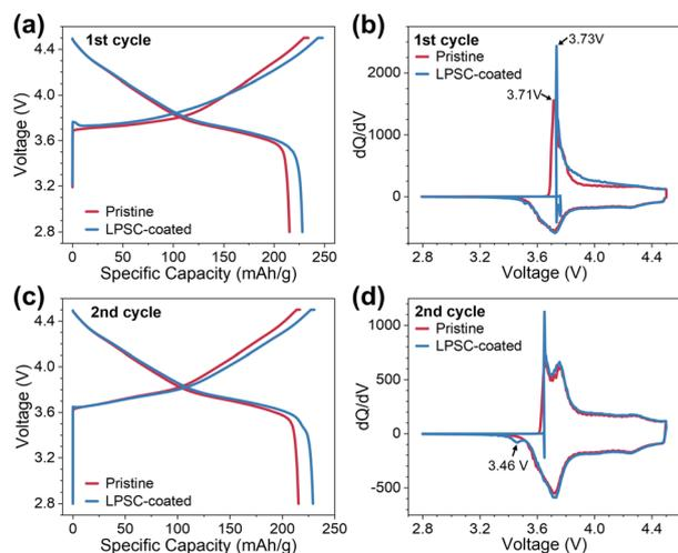
**Fig. 6** (a–d) Voltage profiles and corresponding differential capacity versus  $V$  plots of the pristine and LPSC-coated NMC622 cathodes versus Li electrode cells during two consecutive formation cycles at a cycling rate of C/15.
