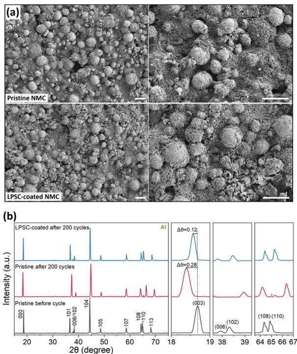
**Fig. 12** (a) HRSEM images of pristine and LPSC-coated NMC622 cathode surfaces after 200 cycles, scalebar: 20  $\mu\text{m}$ . (b) XRD patterns of uncycled the pristine NMC622 cathode and pristine and LPSC-coated cathode after 200 cycles, and magnified view of the (003), (006)/(102), and (108)/(110) reflections.
