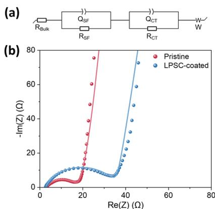
**Fig. 5** (a) The equivalent circuit model for fitting the EIS data. (b) Nyquist plots of EIS measurements and their fits at 30 °C of symmetrical cells comprising uncoated and LPSC-coated NMC622 cathodes.
