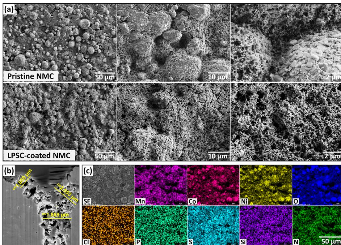
**Fig. 3** (a) HRSEM images of pristine and LPSC-coated NMC622 after deposition at 100 V for 1 min. (b) FIB-HRSEM cross-sectional image of the LPSC + PIL coating layer over the NMC particles. (c) HRSEM and EDS mapping images of LPSC film electrophoretically deposited on NMC622 at 100 V for 1 min.
