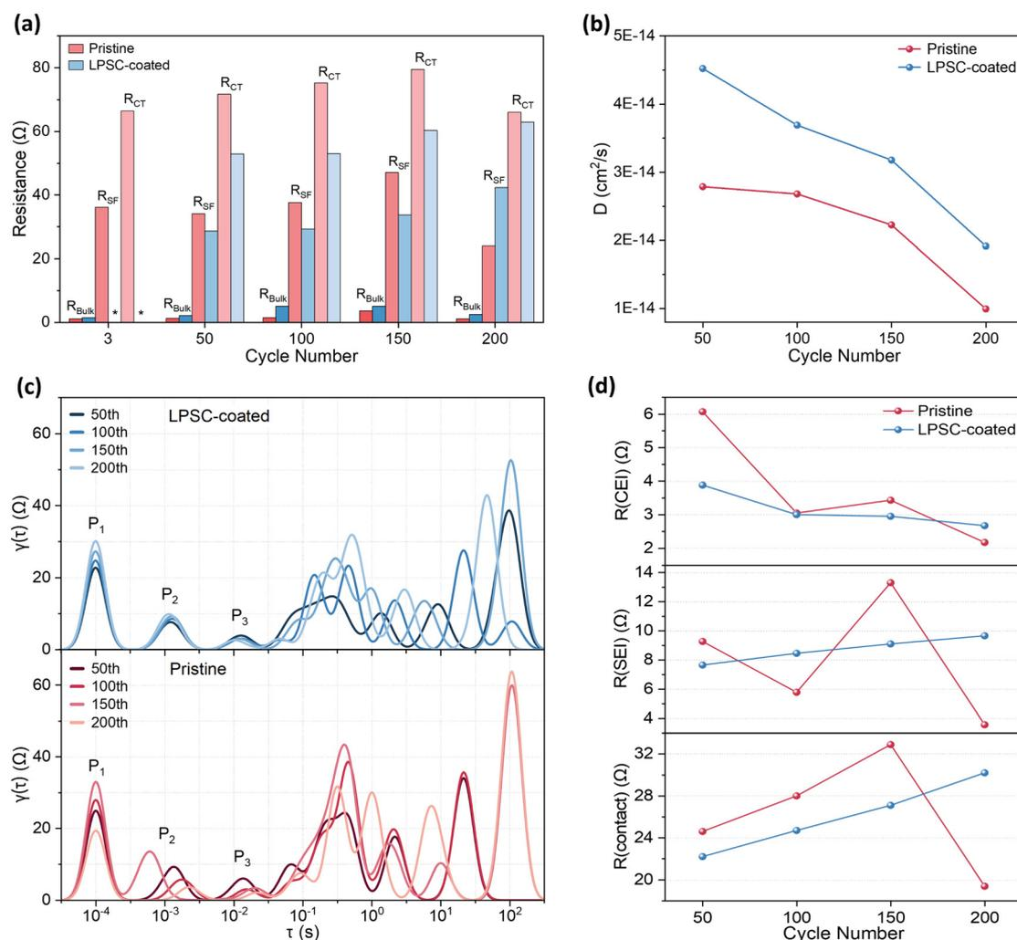
Fig. 9 (a) The fitted resistance values of EIS measurements, (b) the calculated lithium-ion diffusion coefficients, (c) the DRT plots, and (d) the resistances in the intermediate frequency ranges from the DRT plots, during electrochemical cycling after the 50th, 100th, 150th, and 200th cycle at 2.8–4.5 V.
