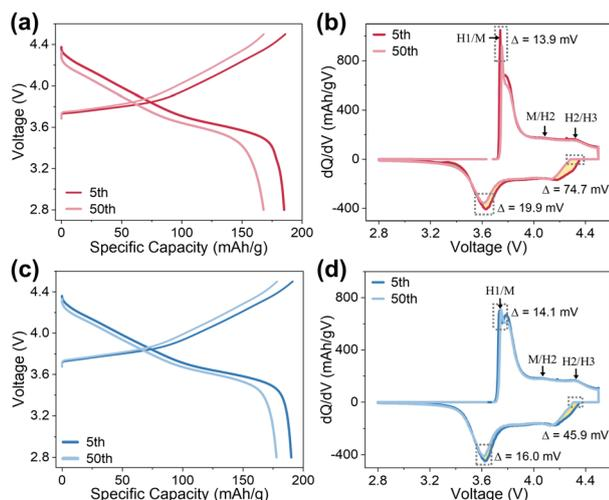
**Fig. 8** Voltage profiles and corresponding differential capacity  $dQ/dV$  versus  $V$  plots for half cells comprising: (a and b) pristine and (c and d) LPSC-coated NMC622 cathodes, at cycles number 5th and 50th.
