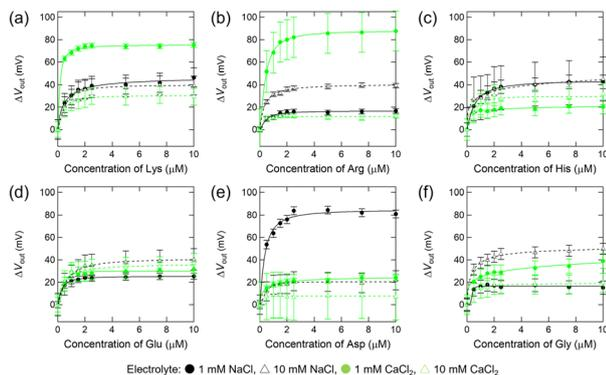
**Fig. 5** Electrical detection of amino acids using the field-effect transistor sensor modified with the cationic monolayer (2-mercaptoethylamine-self-assembled monolayer). Changes in the output voltage upon addition of Lys (a), Arg (b), His (c), Glu (d), Asp (e), or Gly (f) to the 3-morpholinopropanesulfonic acid buffer solution (10 mM) with 1 or 10 mM electrolyte (NaCl or CaCl<sub>2</sub>) at pH 7.0. [Analyte] = 0–10 μM.
