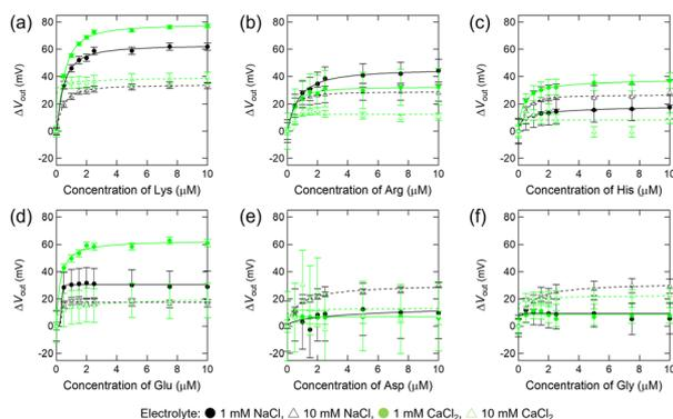
**Fig. 4** Electrical detection of amino acids using the field-effect transistor sensor modified with the anionic monolayer (3-mercaptopropionic acid-self-assembled monolayer). Changes in the output voltage upon addition of Lys (a), Arg (b), His (c), Glu (d), Asp (e), or Gly (f) to the 3-morpholinopropanesulfonic acid buffer solution (10 mM) with 1 or 10 mM electrolyte (NaCl or CaCl<sub>2</sub>) at pH 7.0. [Analyte] = 0–10 μM.
