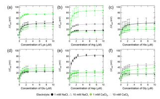
Fig. 5 Electrical detection of amino acids using the field-effect transistor sensor modified with the cationic monolayer (2-mercaptoethylamineself-assembled monolayer). Changes in the output voltage upon addition of Lys (a), Arg (b), His (c), Glu (d), Asp (e), or Gly (f) to the 3-morpholinopropanesulfonic acid buffer solution (10 mM) with 1 or 10 mM electrolyte (NaCl or CaCl<sub>2</sub>) at pH 7.0. [Analyte] =  $0-10 \mu M$ .
