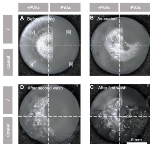
**Fig. 7** PVAc primer layer-mediated coating of silicone implants with the sprayable Coseal hydrogel. Silicone implants were divided into four different zones, visualized by dotted white lines. The images were taken before coating with Coseal (A), immediately after coating (B), and after the first (C), and the second wash (D) with PBS.
