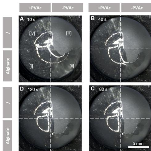
**Fig. 3** PVAc primer layer alters silicone surface properties. Silicone implants were divided into four zones, visualized by dotted white lines. The images were taken at 10 s (A), 40 s (B), 80 s (C), and 120 s (D) after dipping the implants (zone [i] and [iii]) in the alginate solution.
