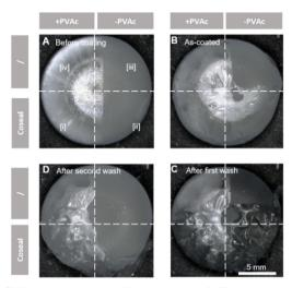
Fig. 7 PVAc primer layer-mediated coating of silicone implants with the sprayable Coseal hydrogel. Silicone implants were divided into four different zones, visualized by dotted white lines. The images were taken before coating with Coseal (A), immediately after coating (B), and after the first (C), and the second wash (D) with PBS.
