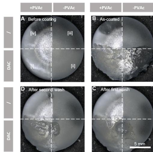
**Fig. 5** PVAc primer layer-mediated coating of silicone implants with a paintable DAC hydrogel. Silicone implants were divided into four zones, visualized by dotted white lines. The images were taken before coating with DAC (A), immediately after coating on zones [i] and [ii] (B), and after the first (C) and the second wash (D) with PBS.
