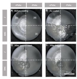
Fig. 5 PVAc primer layer-mediated coating of silicone implants with a paintable DAC hydrogel. Silicone implants were divided into four zones, visualized by dotted white lines. The images were taken before coating with DAC (A), immediately after coating on zones [i] and [ii] (B), and after the first (C) and the second wash (D) with PBS.
